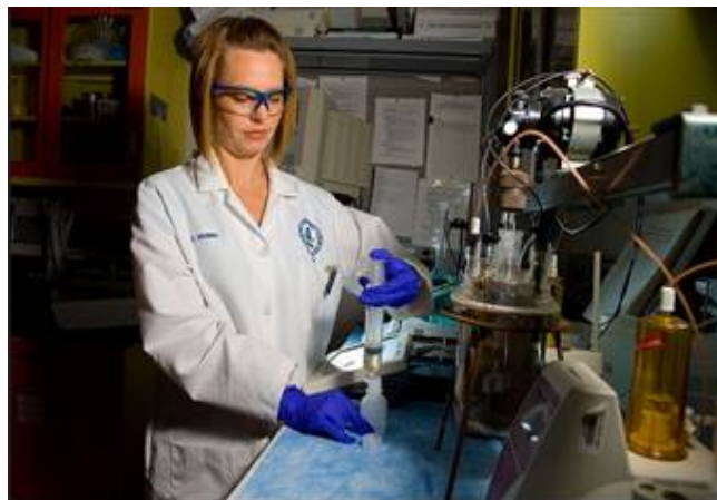
An EPA engineering technician at the Andrew W. Breidenbach Environmental Research Center Lab in Cincinnati synthesizes lead particles to investigate lead corrosion to help develop techniques to prevent lead contamination.
