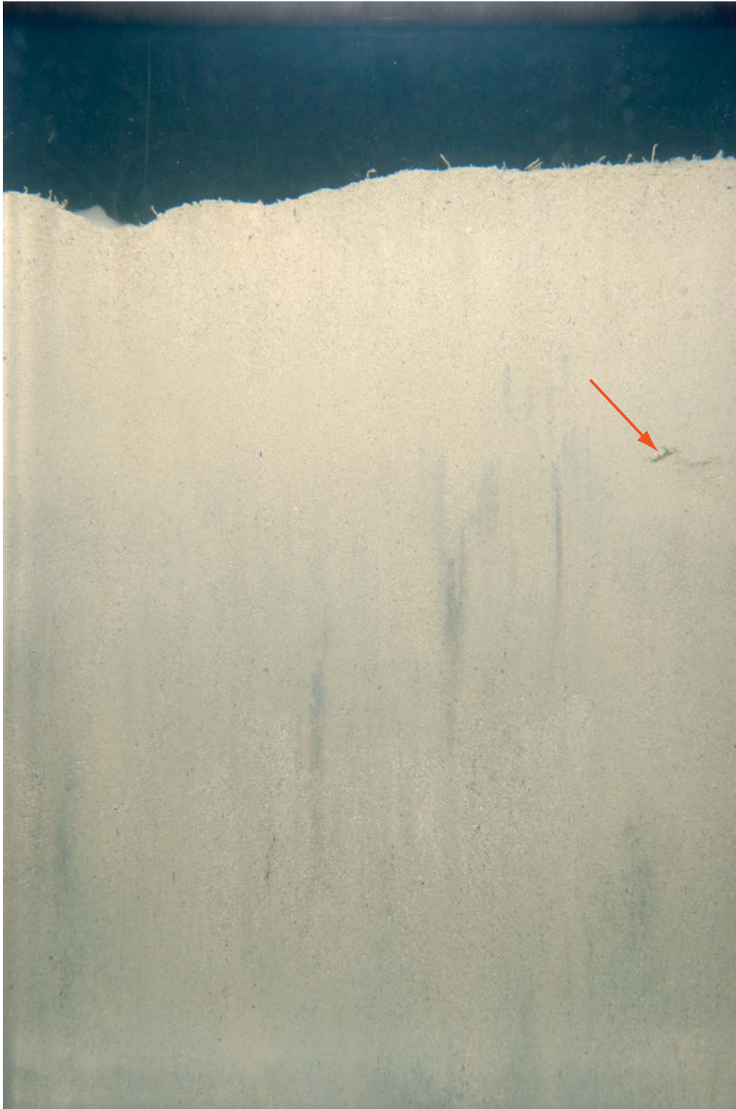
Figure 3-3: SPI image from Station B3 showing typical ambient sediment outside the disposal site consisting of relatively soft, silty, very fine sand (grain size major mode of 4 to 3 phi). Small tubes occur at the sediment surface, and a feeding void is visible at depth (arrow), resulting in a "Stage 1 on 3" successional designation for this image. Scale: actual image width is 14.4 cm.
