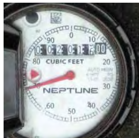
A meter reads 201,670 cubic feet.
