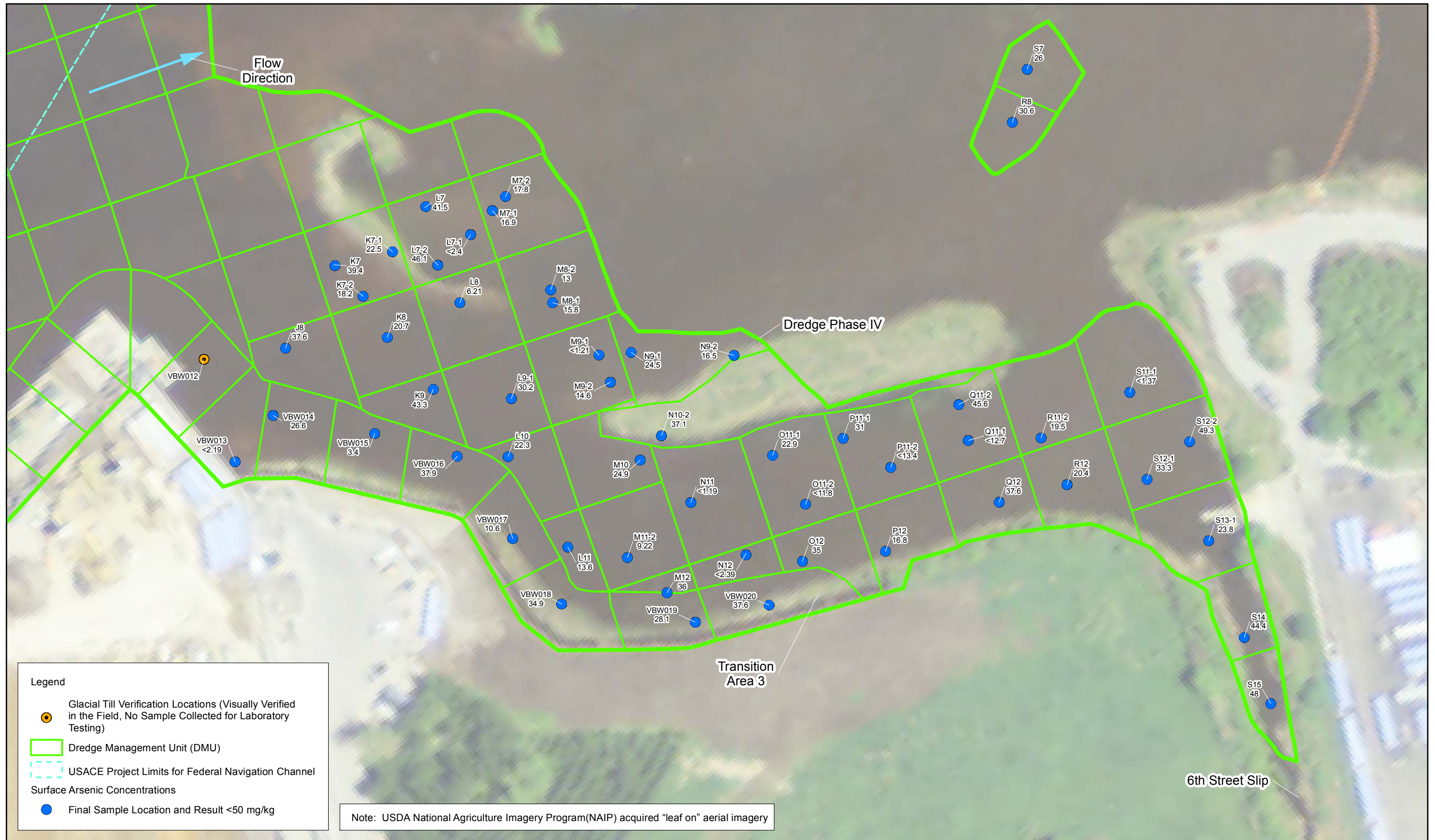
Figure 7 Final Post-Dredge Confirmation Sampling Locations and Results Tyco Fire Products LP Facility Marinette, WI
