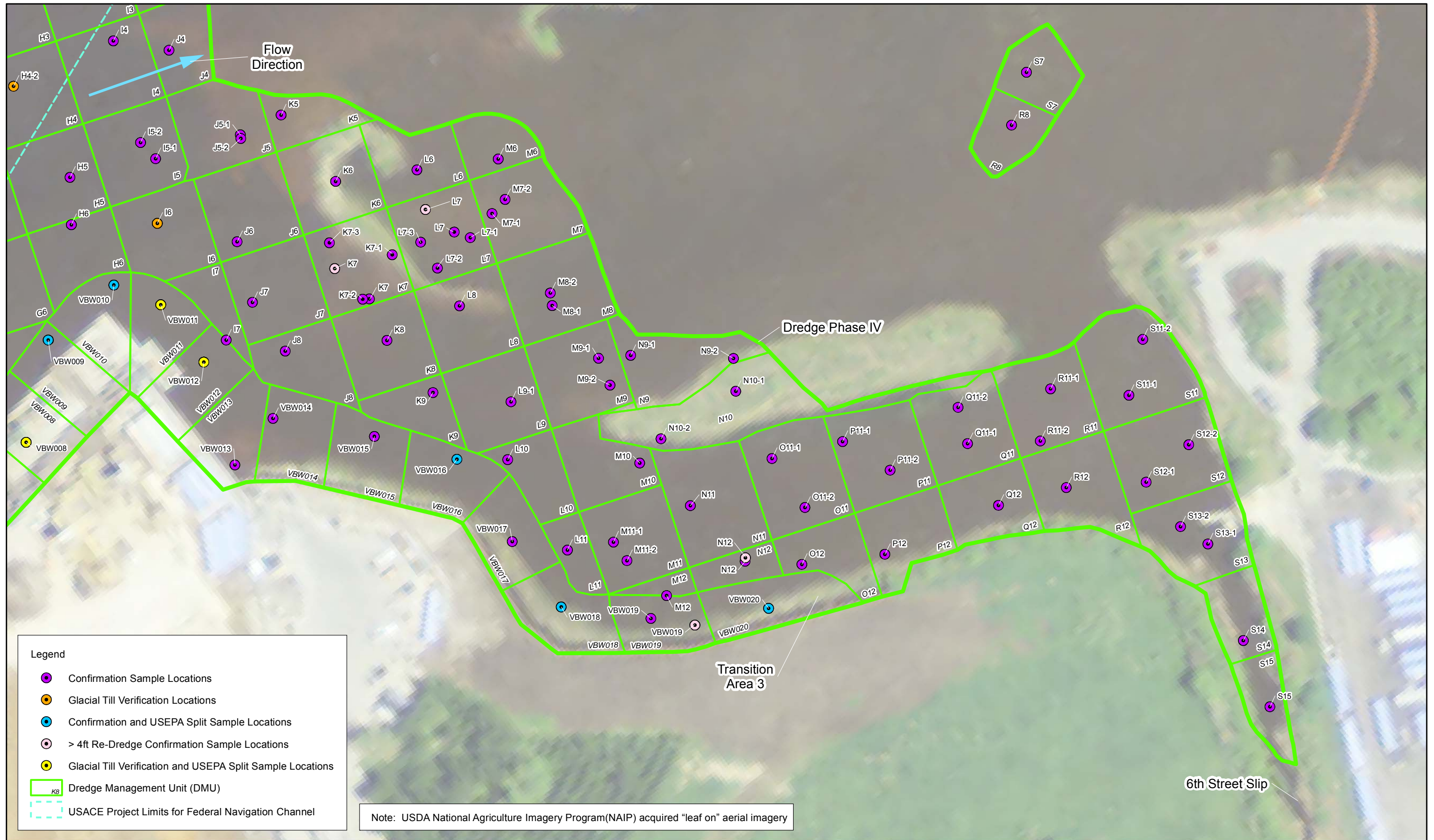
Figure 3 Confirmation Sampling and DMU Locations Tyco Fire Products LP Facility Marinette, WI
