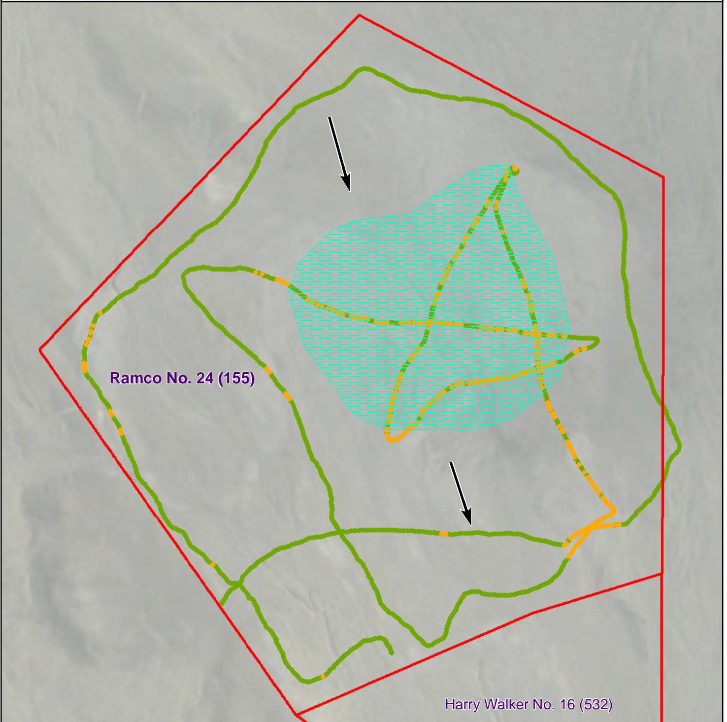
Figure 2 - Gamma Radiation Measurements Ramco No. 24 (155) Coalmine Mesa Chapter, Navajo Nation
