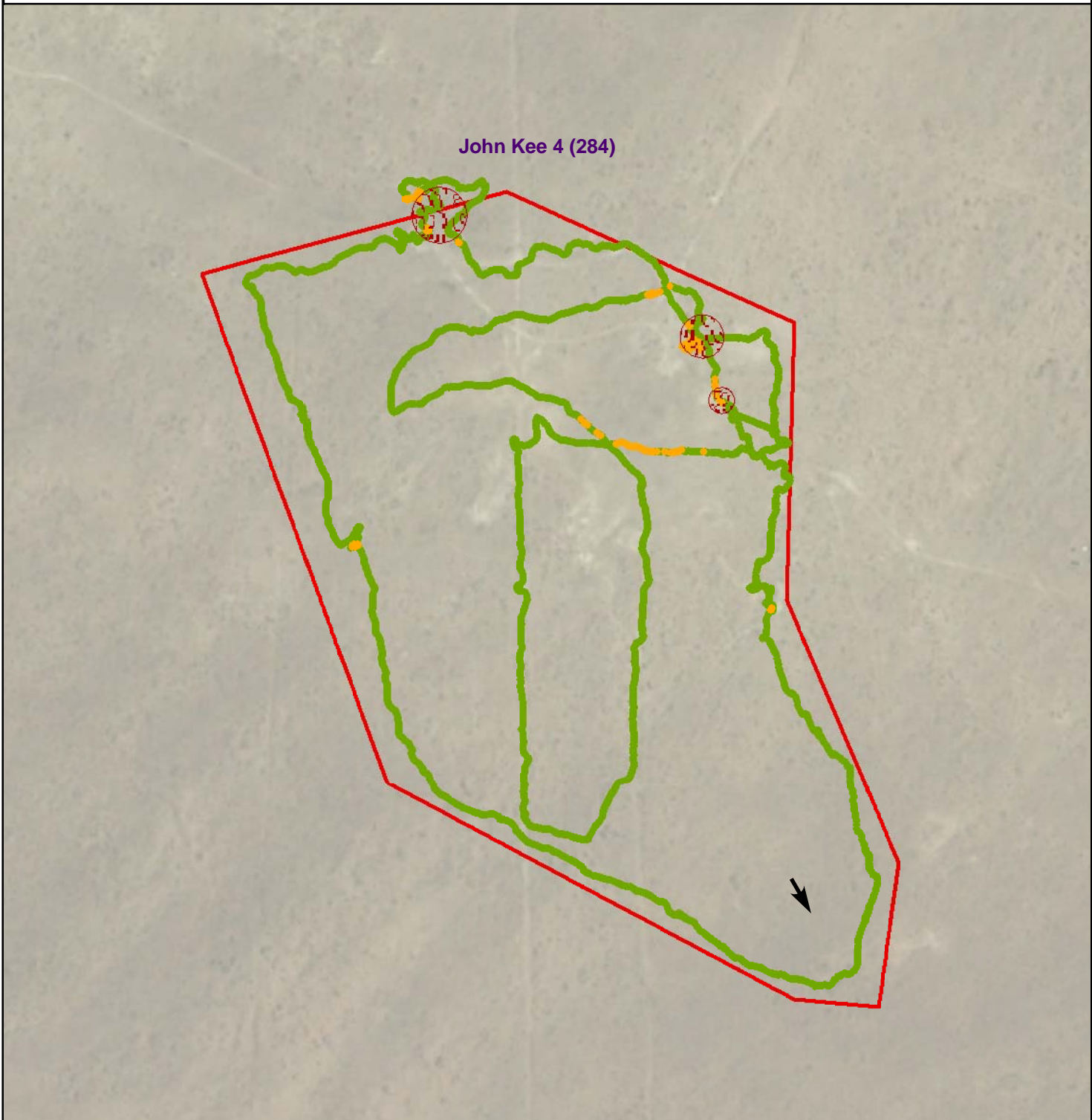
Figure 1 - Gamma Radiation Measurements, Above Two Times Background John Kee 4 (284) Teec Nos Pos Chapter, Navajo Nation
