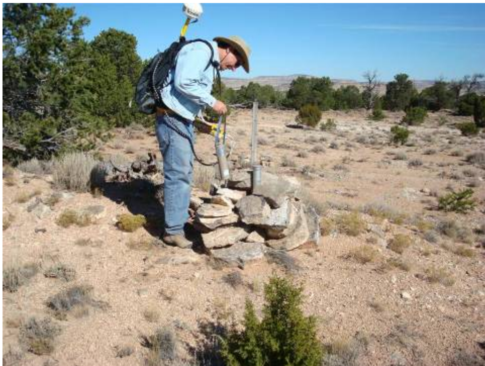
Photo 2. Elkins 326 Mine site, BLM cadastral survey marker
