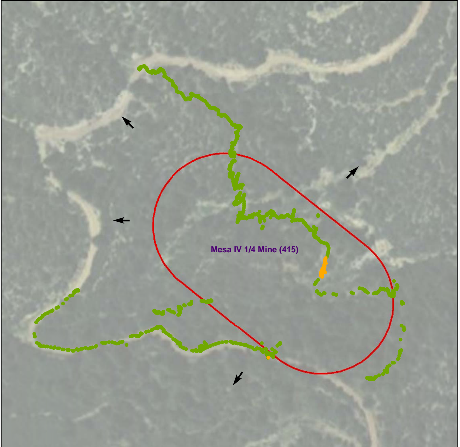
Figure 1 - Gamma Radiation Measurements, Above Two Times Background Mesa IV 1/4 Mine (415) Cove Chapter, Navajo Nation, Arizona
