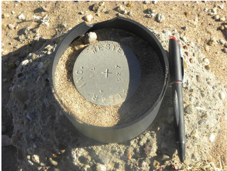
Photo 10. New Liba Group, Site #522, boundary marker
