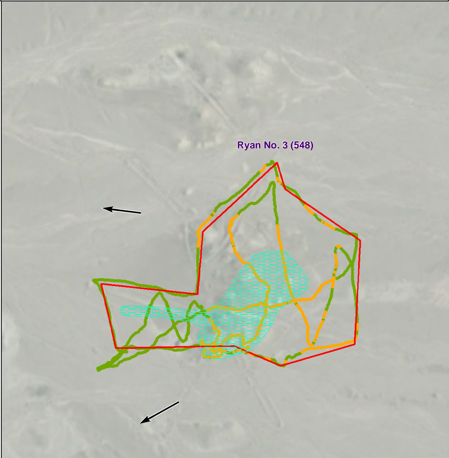
Figure 1 - Gamma Radiation Measurements, Above Two Times Ryan No. 3 (548) Coalmine Mesa Chapter, Navajo Nation
