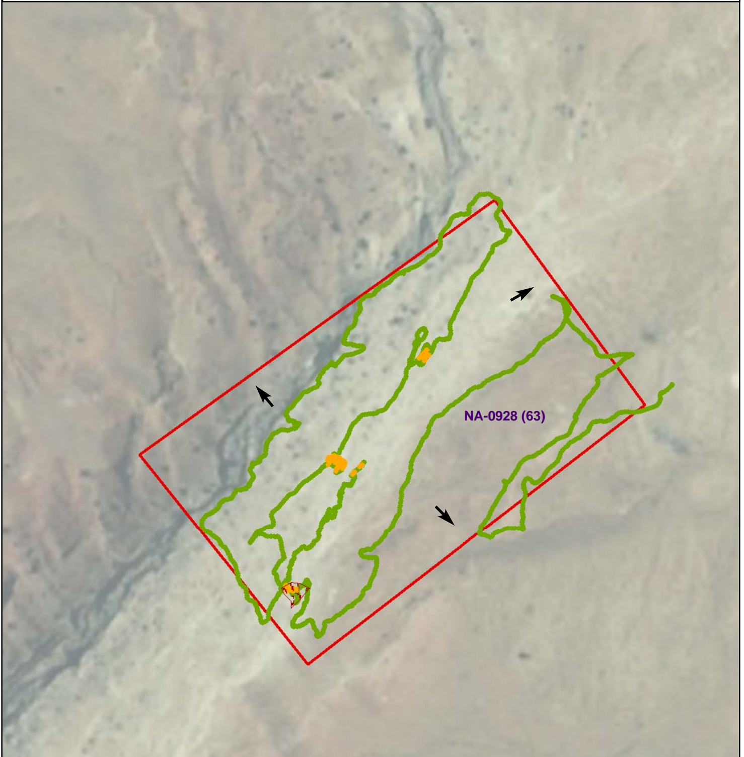
Figure 1 - Gamma Radiation Measurements, Above Two Times Background NA-0928 (63) Teec Nos Pos Chapter, Navajo Nation
