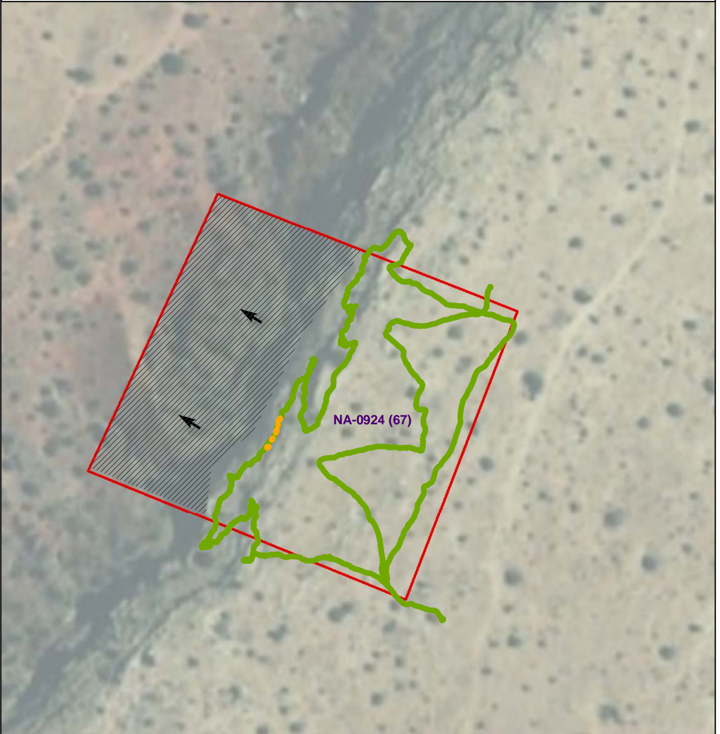
Figure 1 - Gamma Radiation Measurements, Above Two Times Background NA-0924 (67) Sweetwater / Teec Nos Pos Chapter, Navajo Nation
