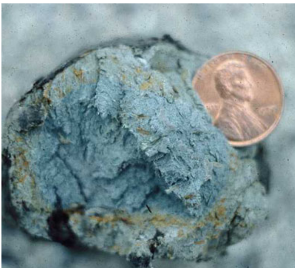
Redoximorphic features (mottling) indicating soil that has been saturated for an extended length of time.
