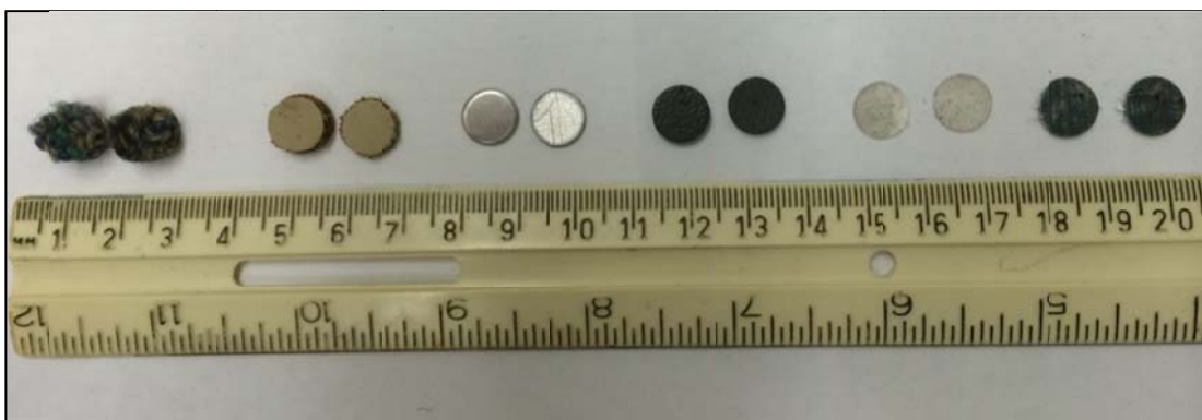
Figure 8. Material coupons (from left to right): nylon loop-pile carpet, fiberglass wall paneling, aluminum, rubber flooring, Mylar® on polycarbonate, and vinyl seating
