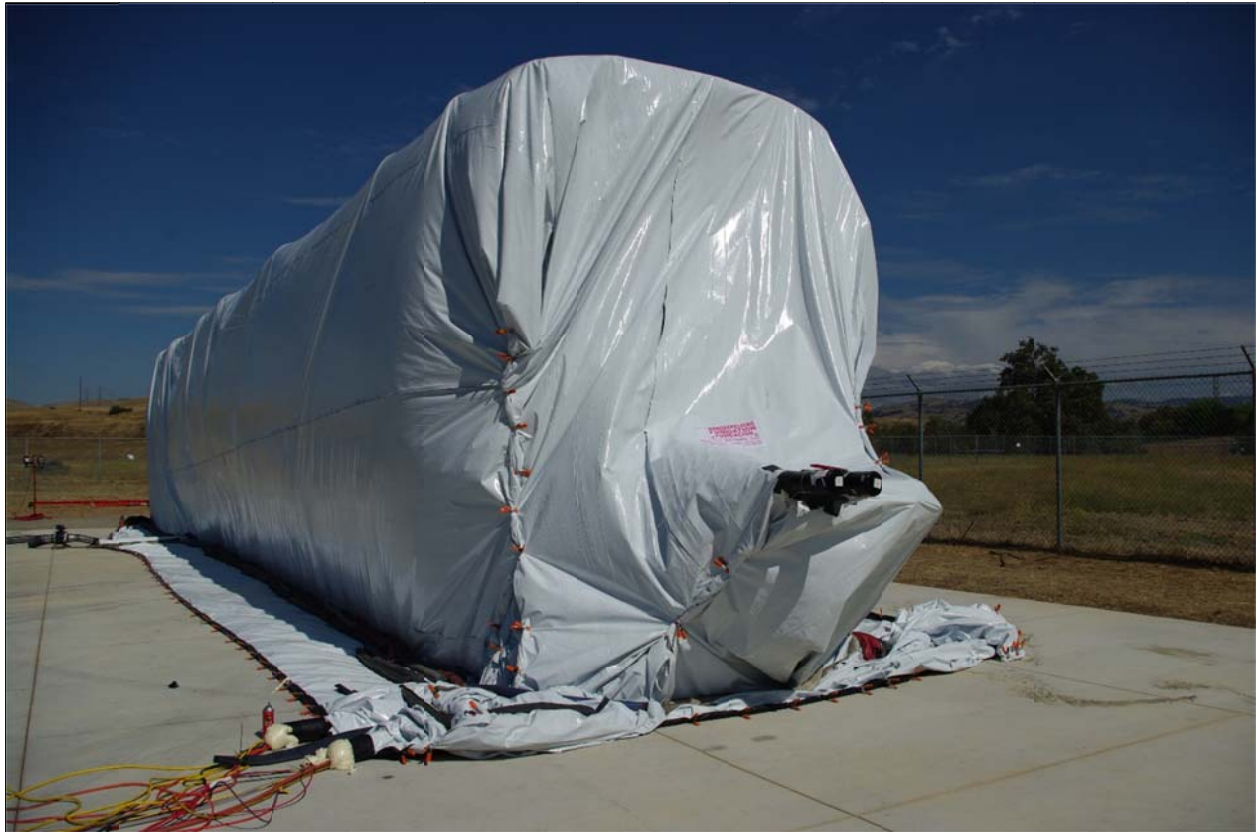
Figure 4. Termini of PVC piping used for timed-series coupon extractions
