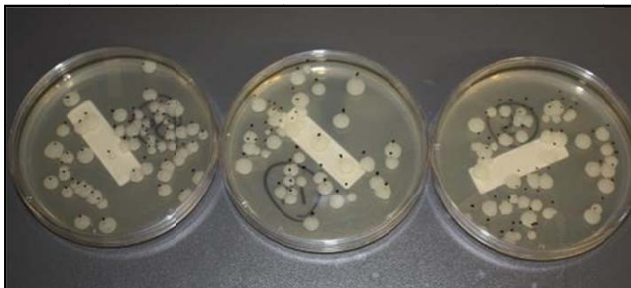
Figure 12. Representative dilution plates after incubation containing Ba Sterne strain spore colonies recovered from coupons
