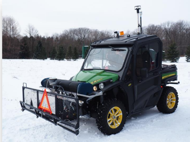
NETL's Utility Terrain Vehicle (UTV) equipped with methane detection instrumentation
