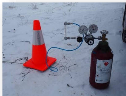
Controlled CH 4 release
