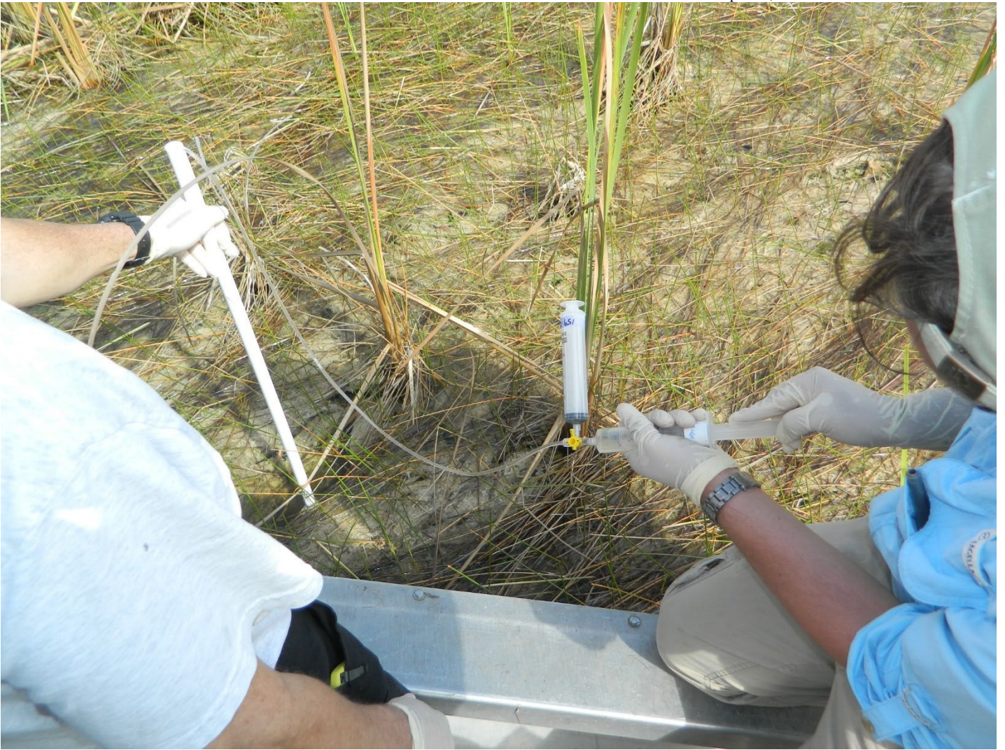
Figure 2. Valve and syringes assembly Valve and syringes assembly attached to sampler in place. Purging shown.
