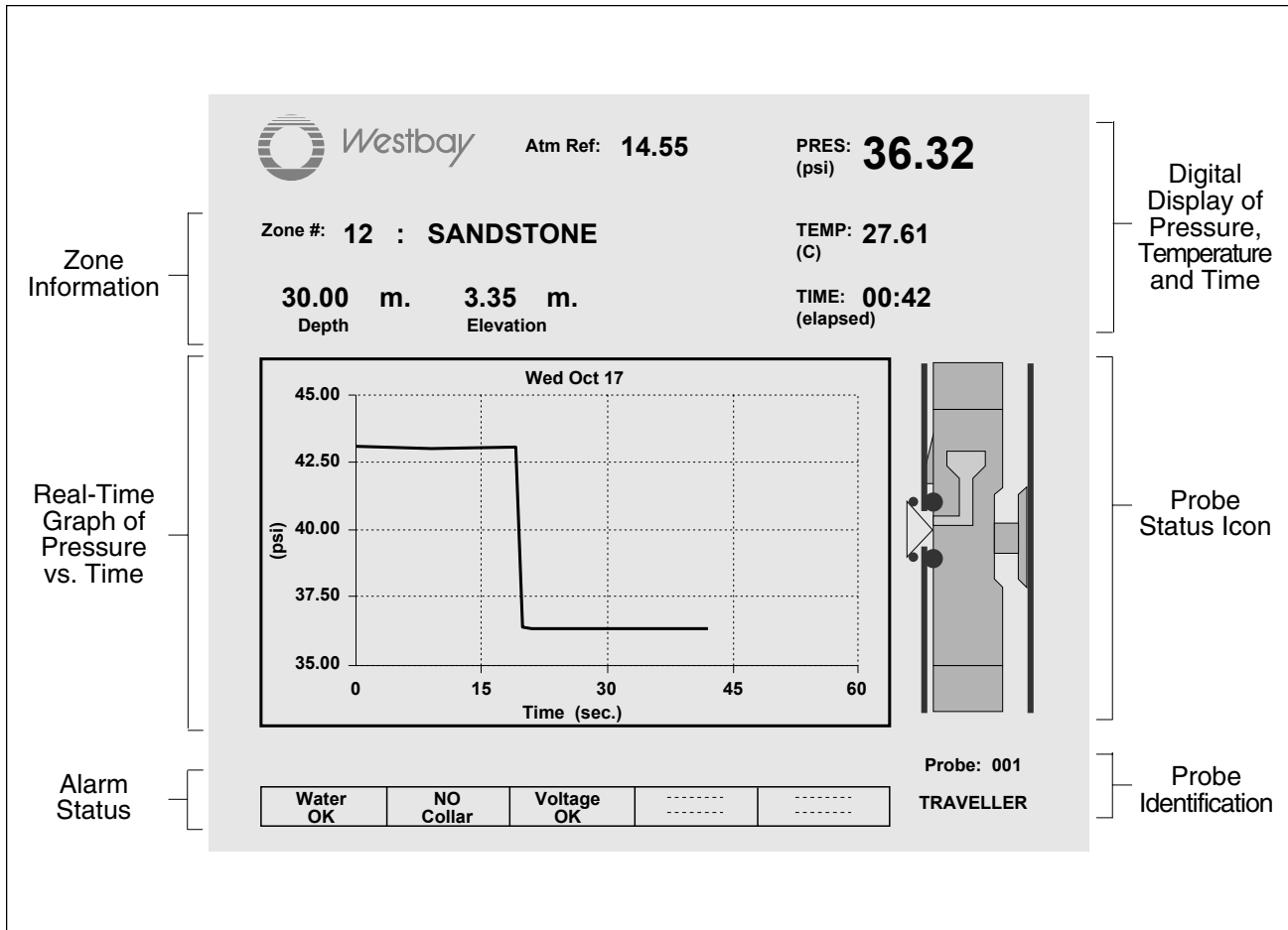
Figure 8. Data display on surface computer when using MProfile software to operate a MOSDAX pressure probe.
