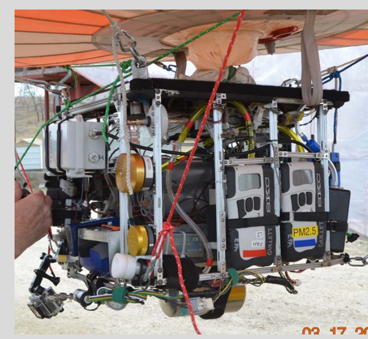
The 46 lb [21 kg] sampling package called the “Flyer”.
