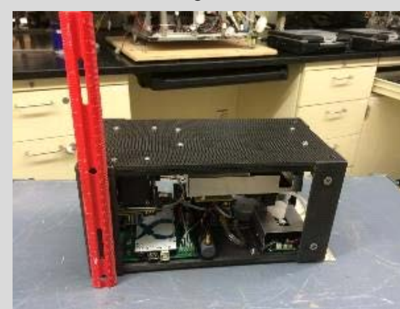
6-11 lb [3-5 kg] sampling package called the “Kolibri” (L) and its internals (R).
