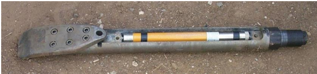
Exhibit A-9. Typical Drillhead (With Cavity Open)
