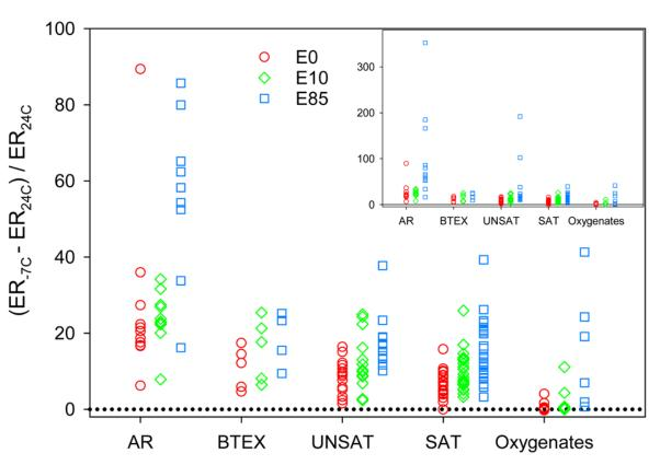
Cold temp VOC emissions enhancements vary with compound class and fuel
