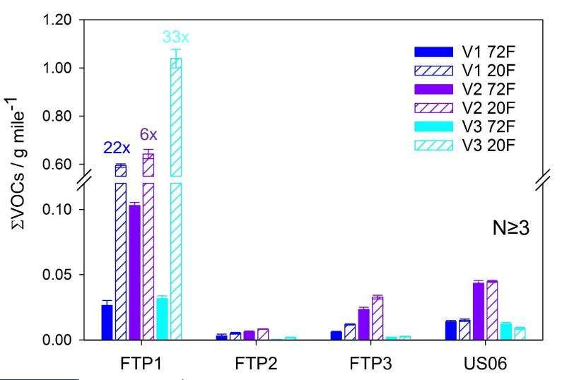
Cold start emissions were substantially higher (4-400x) than warm start (intensified at 20F)
