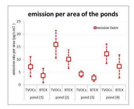
VOCs =  $10\pm 6 \mu g/s \text{ per m2}$ BTEX =  $5\pm 3 \mu g/s \text{ per m2}$
