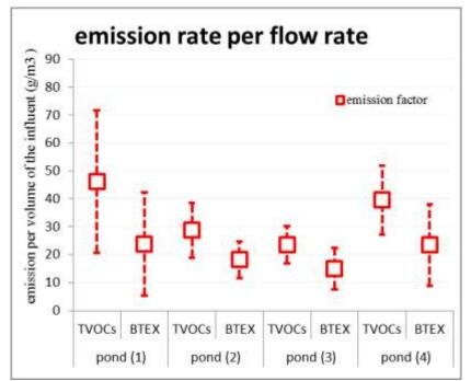
VOCs =  $34\pm 8 \text{ g/m}^3$ BTEX =  $20\pm 3 \text{ g/m}^3$
