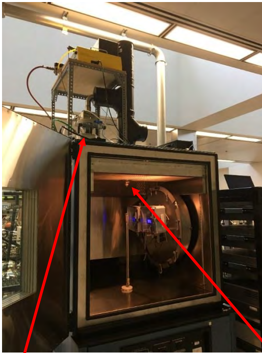
Artificial Aerosol Generation System, AGK PALAS 2000
