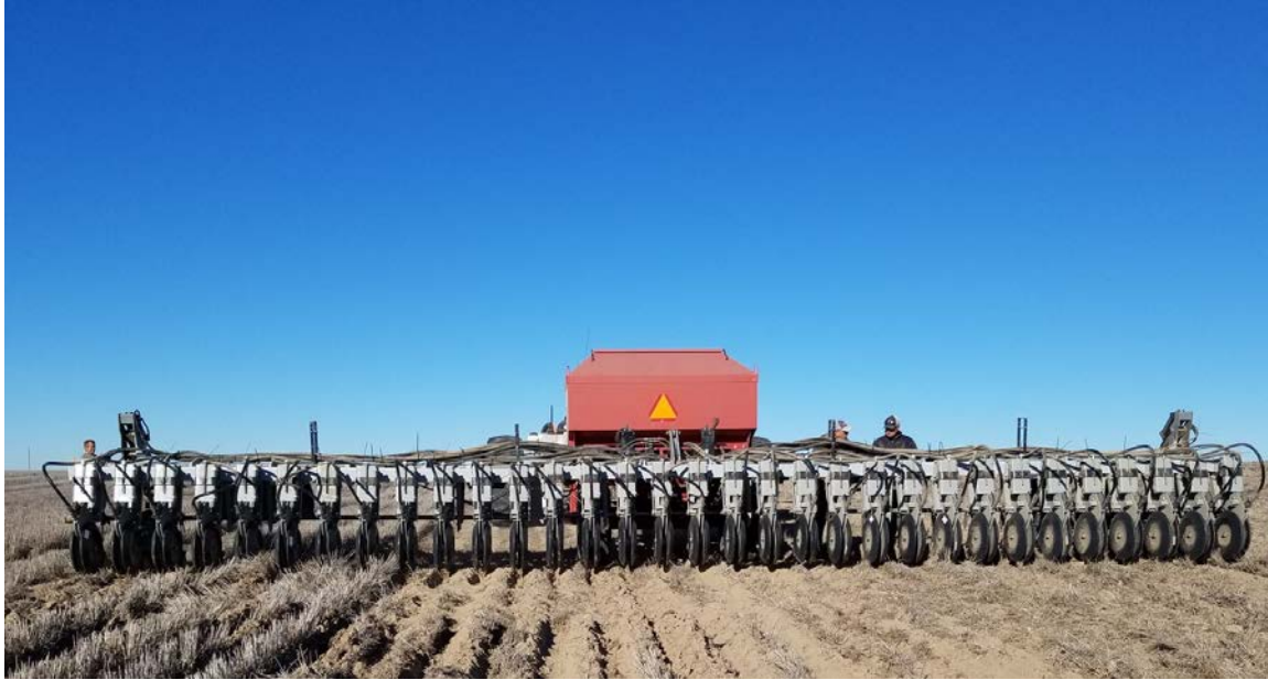
Figure 34. Deep furrow conservation drill prototype (photo credit – Samantha Crow, WSU Lind Research Station)
