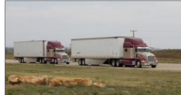
Platooning reduces aerodynamic drag by decreasing the driving distance between vehicles.
