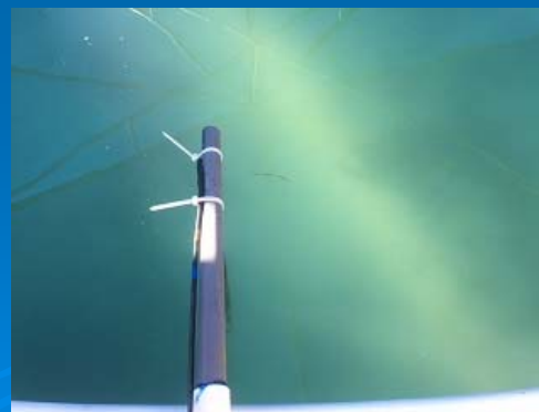
Raw water from New Pass Mesocosm pre-ozone ORP = 300 mv
