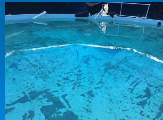
Ozone treated Mesocosm ORP to 750 mv in 7 hrs
