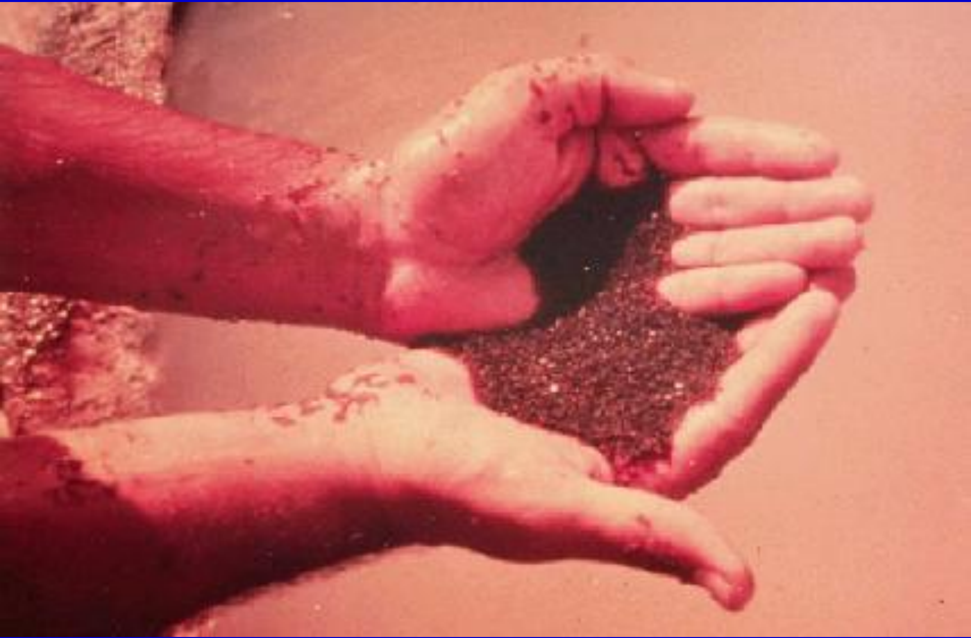
Ion exchange resin beads used in the ISR process
