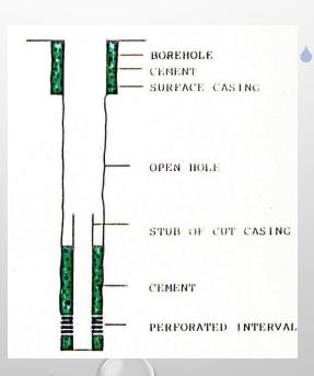
If cement voids or other loss of cement integrity is suspected, squeeze cementing may be necessary
