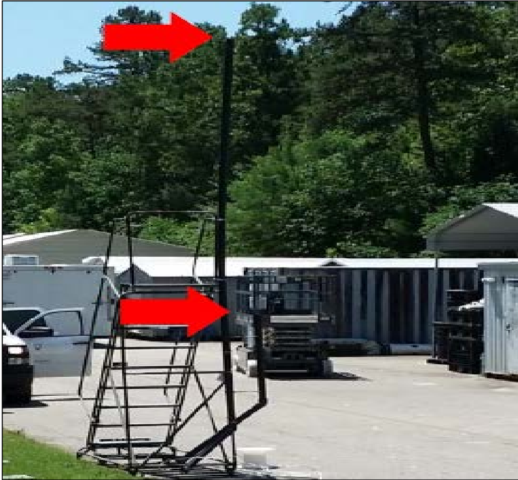
Figure 3-41. High/Low Controlled Gas Release Platform
