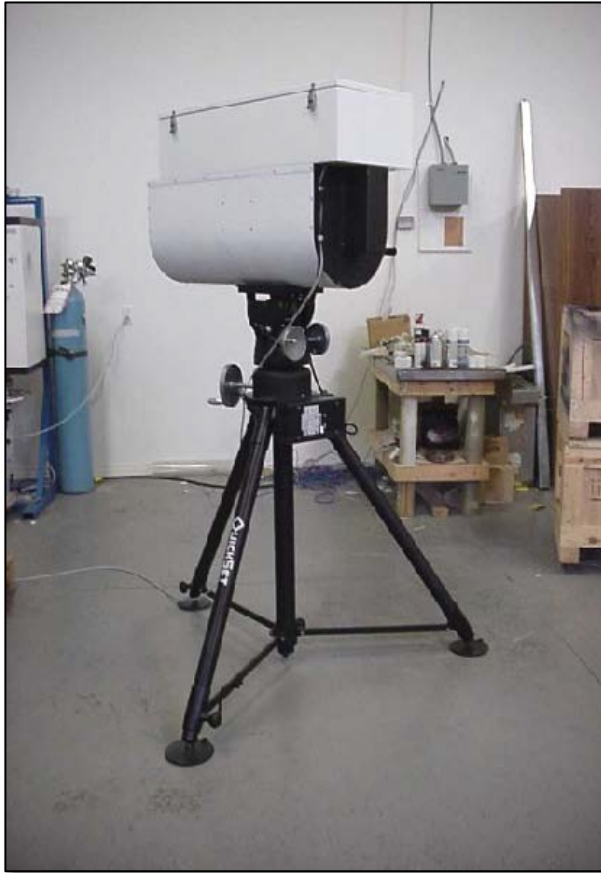
Figure 2-6 Typical telescopic FTIR Transmitting and Detection Unit
