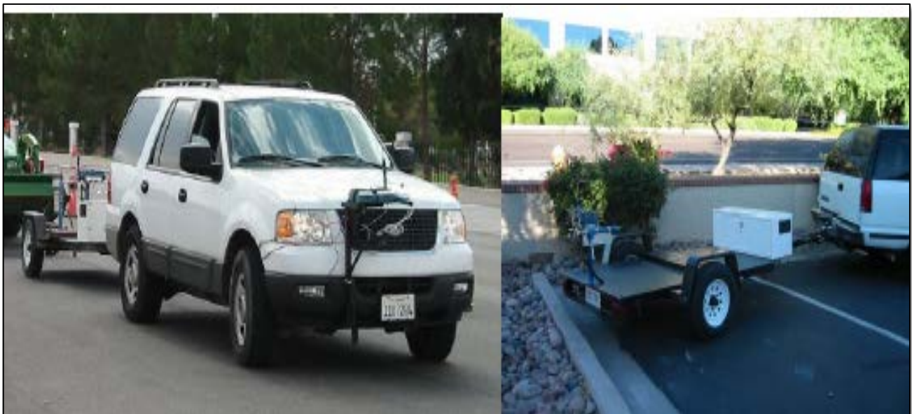
Figure 3.57. Sample inlet installation on a trailer pulled behind the test vehicle.
