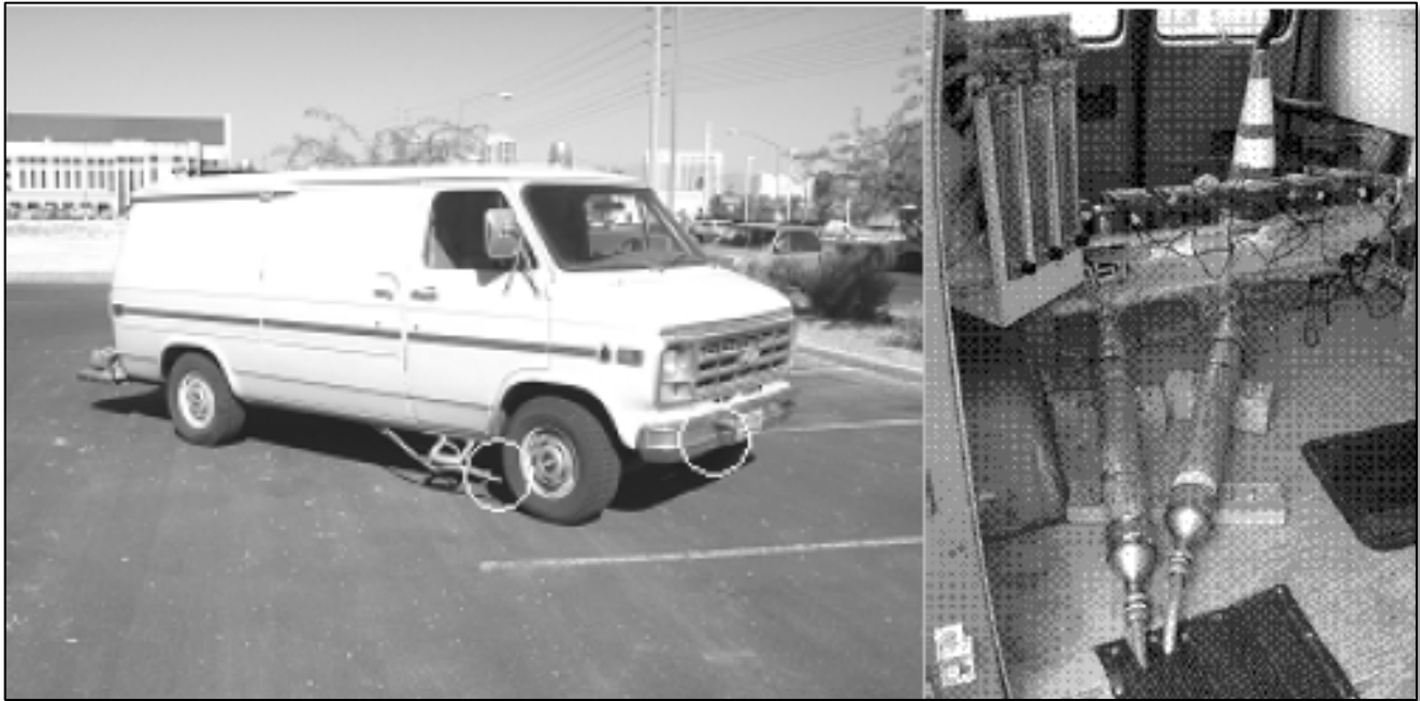
Figure 3-56: Sample inlet installation behind the front tire.
