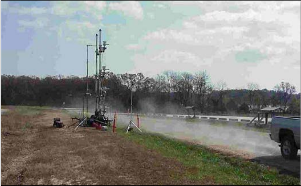
Figure 3.55. deployment of Collocated Plume Profiling Towers at Roadside Location.
