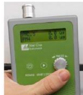
A hand-held air monitor that measures particulate matter in the air. (EPA photo)
