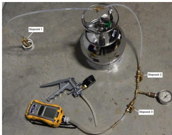
Figure 1. Example of Sub-Slab Sampling and Leak-Test Setup
