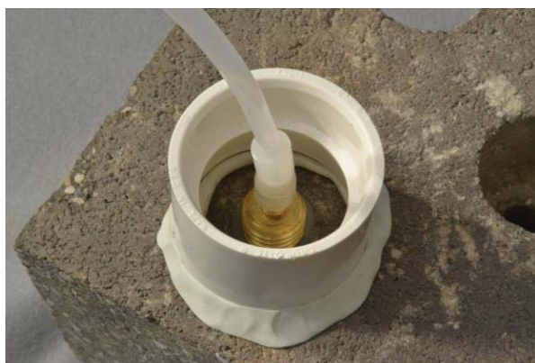
Figure 6. Water dam used for leak detection
