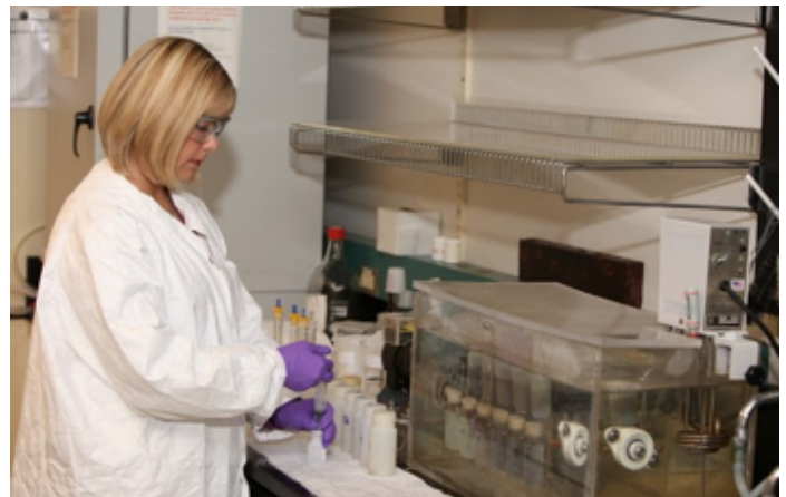
EPA researcher Karen Bradham uses a “virtual stomach” that mimics human digestion to determine if lead and arsenic in contaminated soils are bioavailable.
