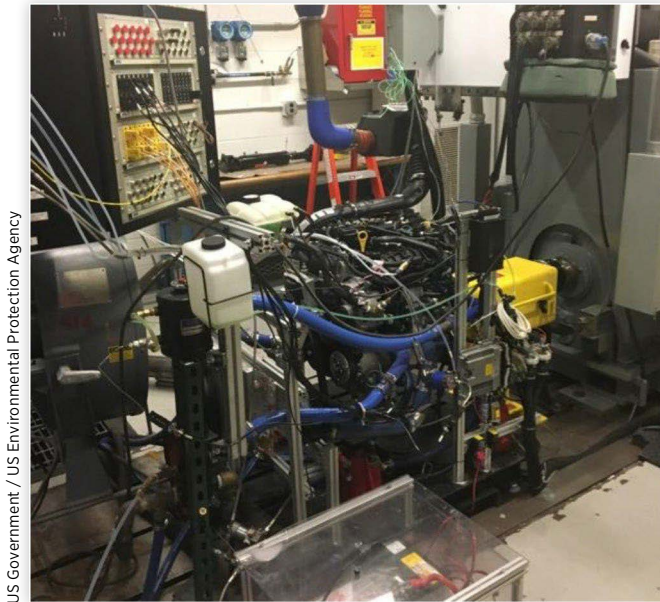
FIGURE 10 Ford 1.6 L EcoBoost engine installed at EPA test facility
