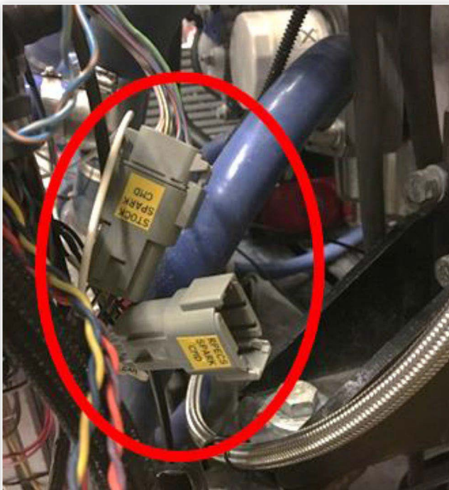
FIGURE 2 Wiring harness modifications for ignition SIC
