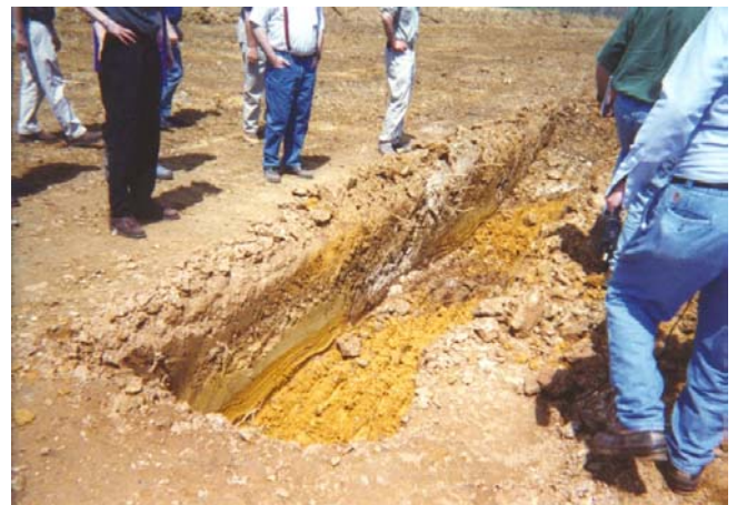
FIGURE 1 EXCAVATED CROSS-SECTION OF BIOSOLIDS TRENCH
