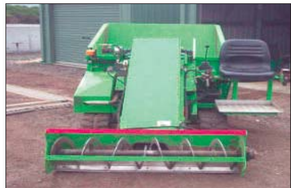
Dried Solids Harvesting Unit
