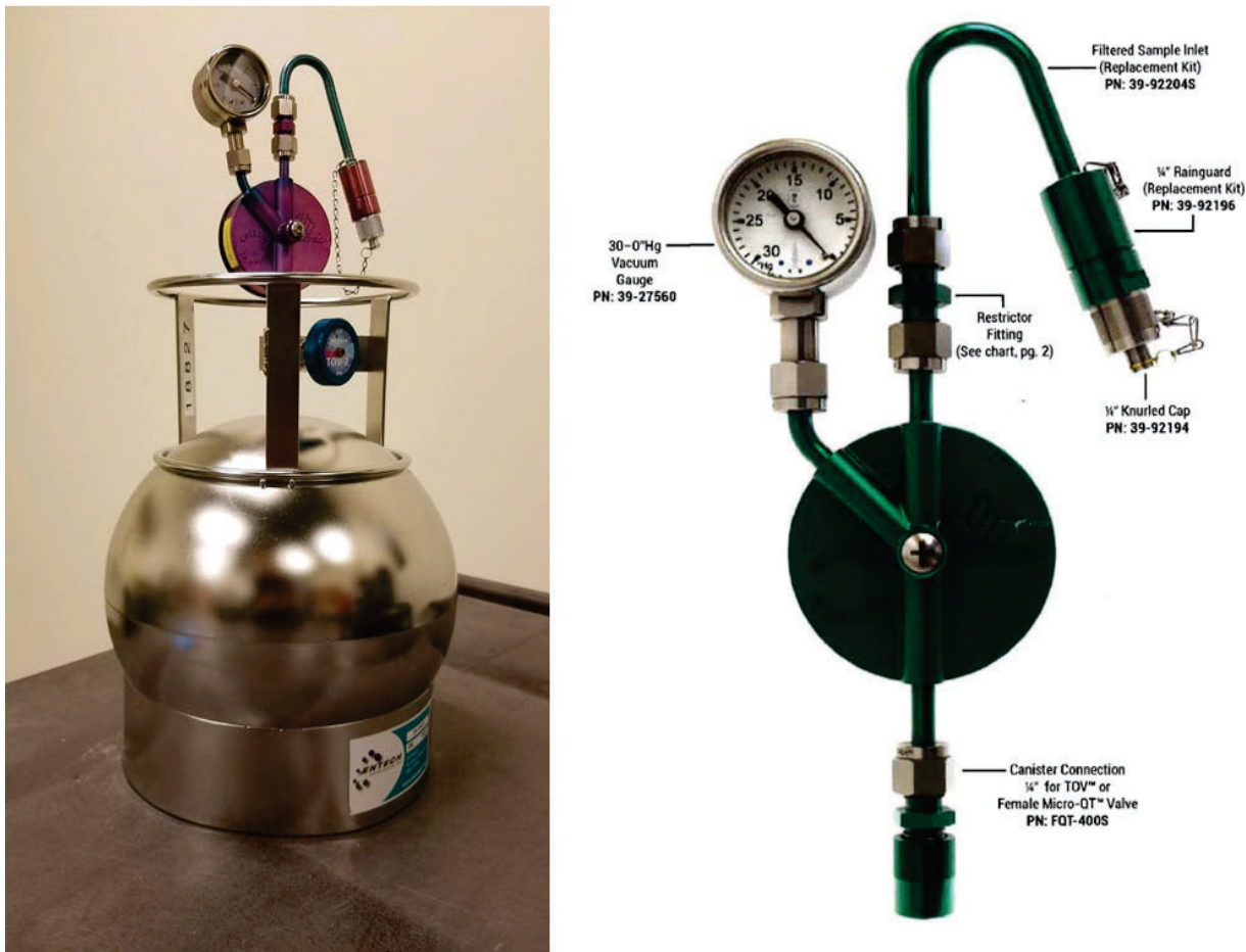
Figure 2-7. Canister setup with Passive Vacuum Regulator.
