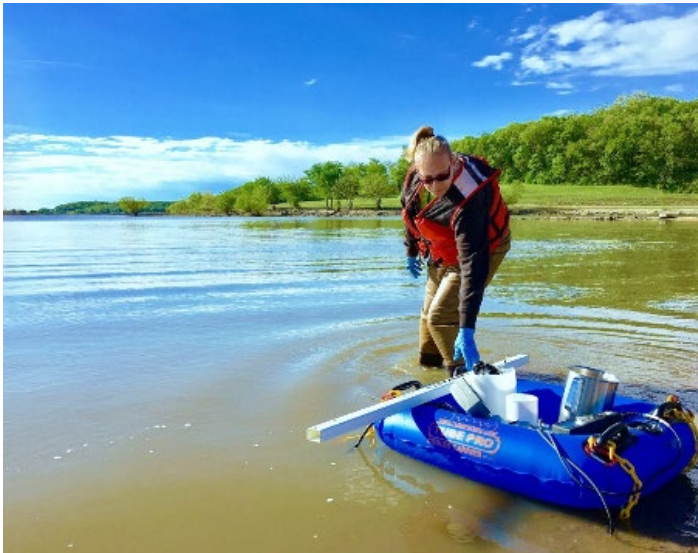
Photo 2: Deanna Collier, Environmental Sciences and Technology Division, carefully takes sampling equipment onto Perry Lake for collection of water samples. She collected water at depths of 1/3 meter, 2/3 meter, and 1 meter. She also ran and recorded information from the monitoring device that collects certain physical and chemical data, such as temperature, pH, and dissolved oxygen.
