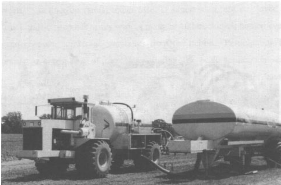
Figure 5-1. Storage tank and application vehicle.
