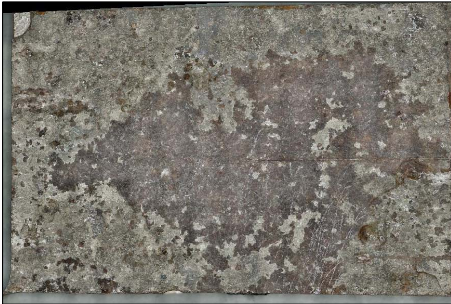
Figure 159. A screenshot of the 3D digital image of a specimen excised from Coupon 5 labeled as 5-2, after CO 2 blast cleaning
