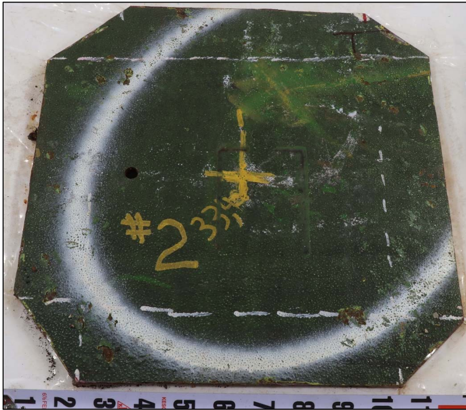
Figure 5. An image of the exterior surface of Coupon 2 in the as-received condition.
