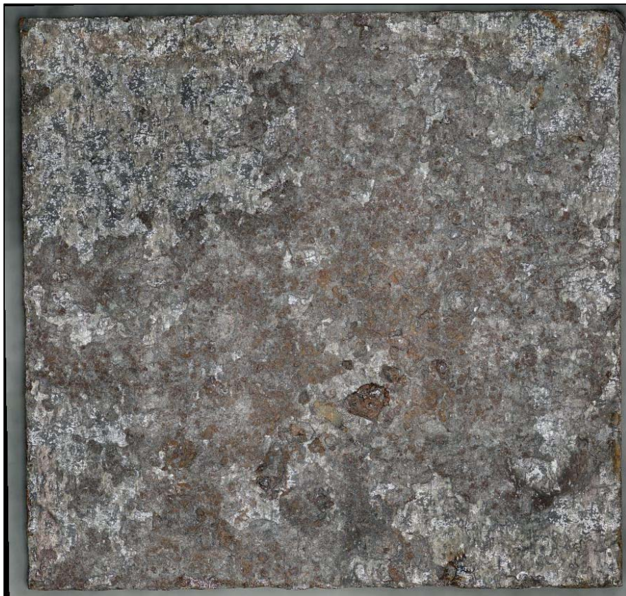
Figure 170. A screenshot of the 3D digital image of a specimen excised from Coupon 8 labeled as 8-3, after CO 2 blast cleaning
