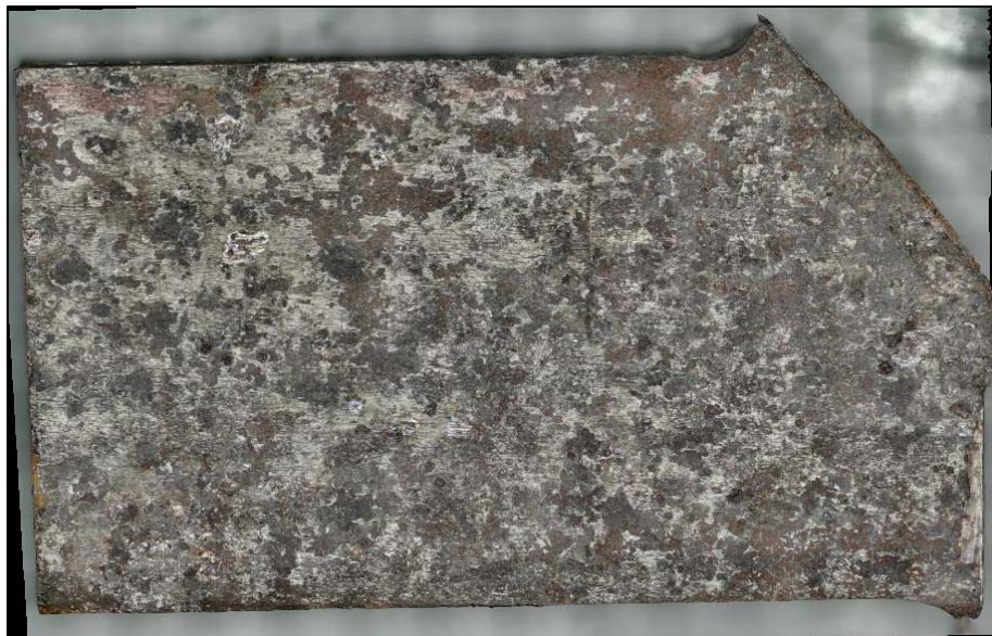
Figure 168. A screenshot of the 3D digital image of a specimen excised from Coupon 8 labeled as 8-1, after CO 2 blast cleaning
