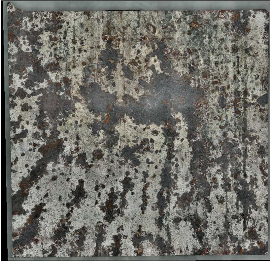
Figure 149. A screenshot of the 3D digital image of a specimen excised from Coupon 1 labeled as 1-1, after CO 2 blast cleaning
