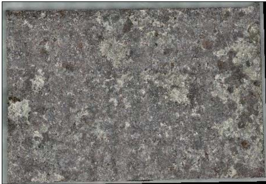
Figure 178. A screenshot of the 3D digital image of a specimen excised from Coupon A-2 labeled as A2-2, after CO 2 blast cleaning
