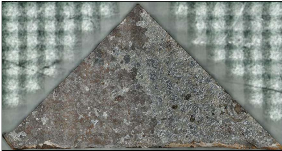
Figure 169. A screenshot of the 3D digital image of a specimen excised from Coupon 8 labeled as 8-2, after CO 2 blast cleaning
