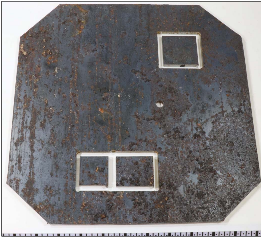
Figure 129. An image of the interior surface of Coupon 1 after CO 2 blast cleaning.
