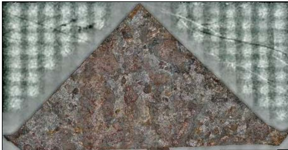
Figure 176. A screenshot of the 3D digital image of a specimen excised from Coupon A-1 labeled as A1-3, after CO 2 blast cleaning
