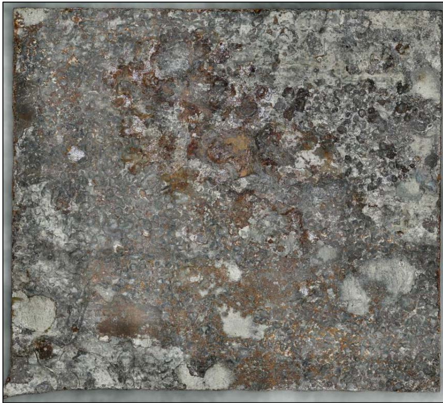
Figure 175. A screenshot of the 3D digital image of a specimen excised from Coupon A-1 labeled as A1-2, after CO 2 blast cleaning
