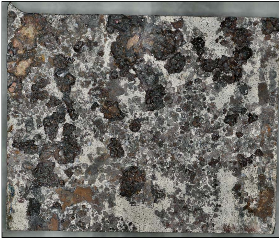
Figure 151. A screenshot of the 3D digital image of a specimen excised from Coupon 1 labeled as 1-3, after CO 2 blast cleaning
