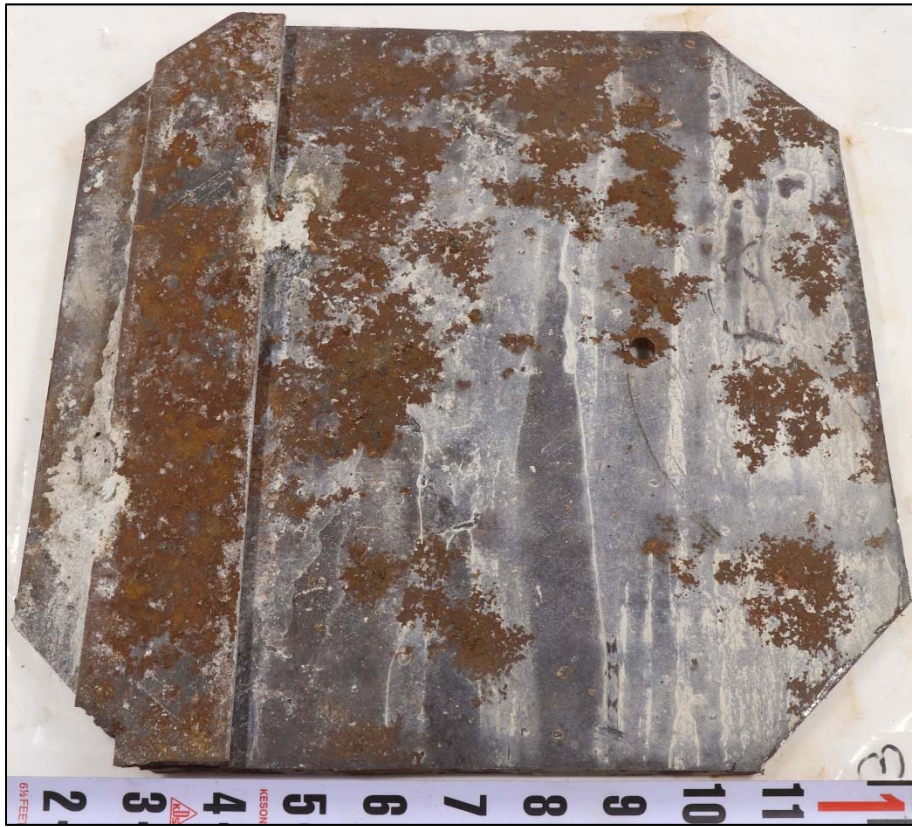
Figure 19. An image of the interior surface of Coupon 8 in the as-received condition.
