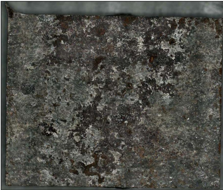
Figure 158. A screenshot of the 3D digital image of a specimen excised from Coupon 5 labeled as 5-1, after CO 2 blast cleaning
