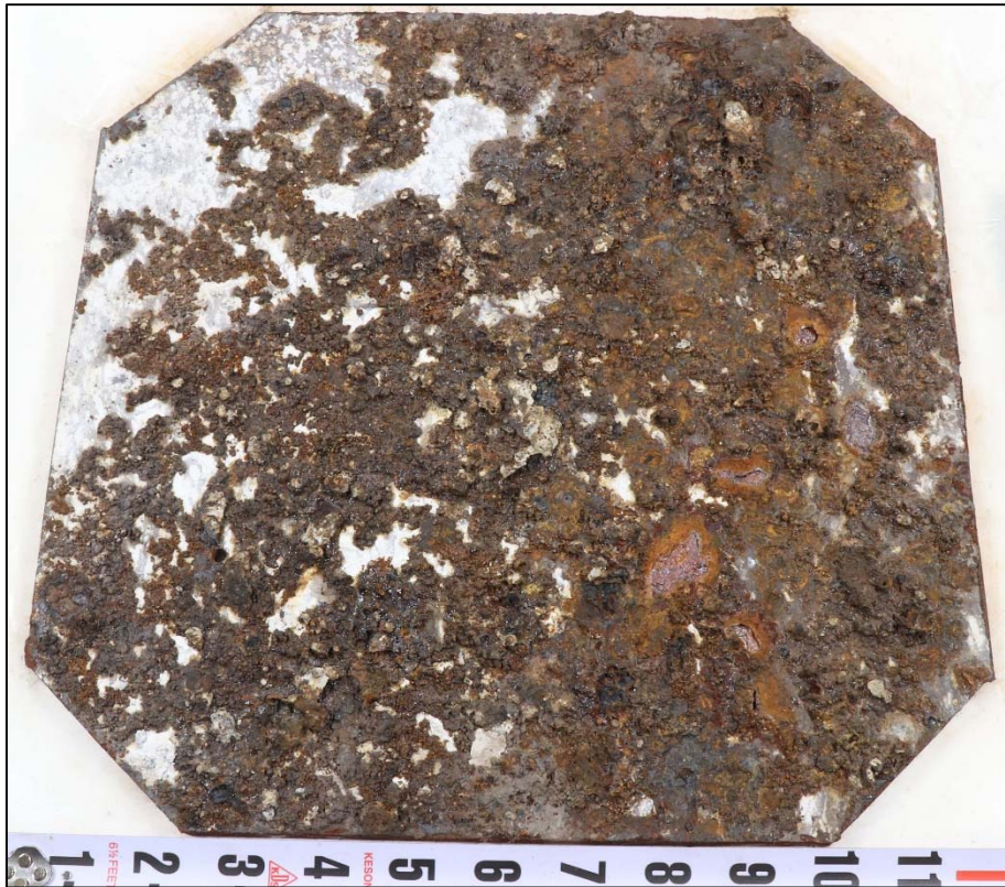
Figure 16. An image of the interior surface of Coupon 7 in the as-received condition.
