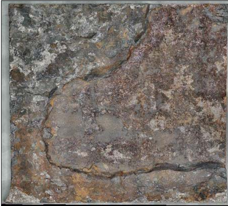
Figure 153. A screenshot of the 3D digital image of a specimen excised from Coupon 2 labeled as 2-2, after CO 2 blast cleaning
