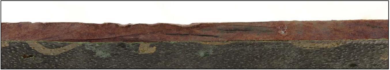
Figure 21. An image of a representative edge of Coupon 8 in the as-received condition.
