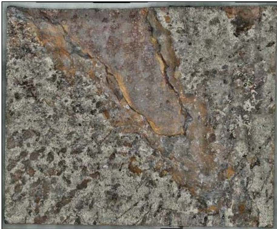
Figure 152. A screenshot of the 3D digital image of a specimen excised from Coupon 2 labeled as 2-1, after CO 2 blast cleaning
