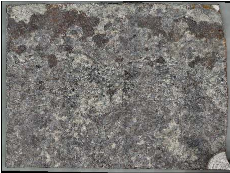
Figure 179. A screenshot of the 3D digital image of a specimen excised from Coupon A-2 labeled as A2-3, after CO 2 blast cleaning
