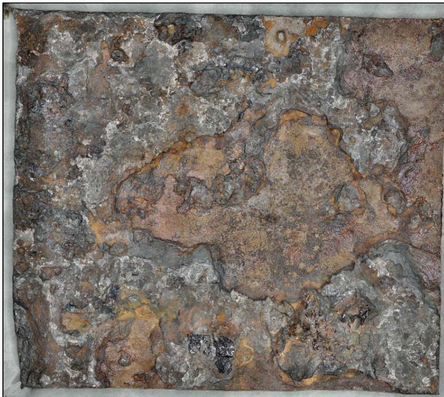
Figure 164. A screenshot of the 3D digital image of a specimen excised from Coupon 7 labeled as 7-1, after CO 2 blast cleaning
