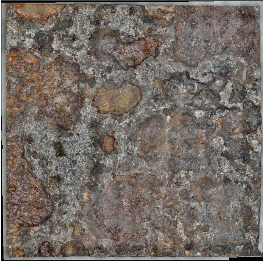
Figure 165. A screenshot of the 3D digital image of a specimen excised from Coupon 7 labeled as 7-2, after CO 2 blast cleaning.
