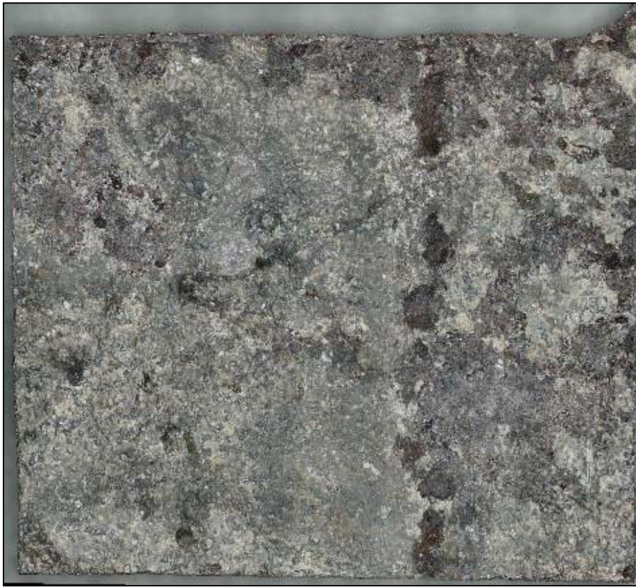
Figure 177. A screenshot of the 3D digital image of a specimen excised from Coupon A-2 labeled as A2-1, after CO 2 blast cleaning
