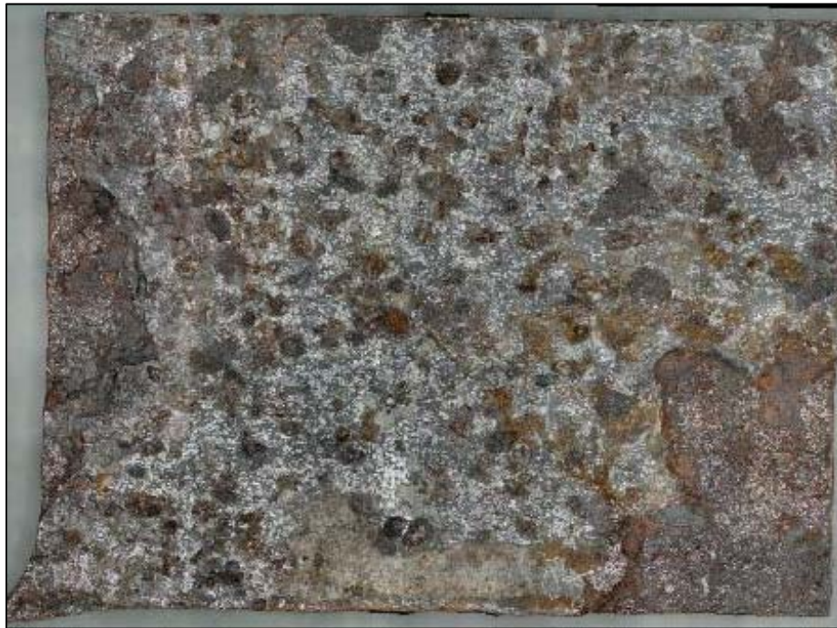
Figure 174. A screenshot of the 3D digital image of a specimen excised from Coupon A-1 labeled as A1-1, after CO 2 blast cleaning
