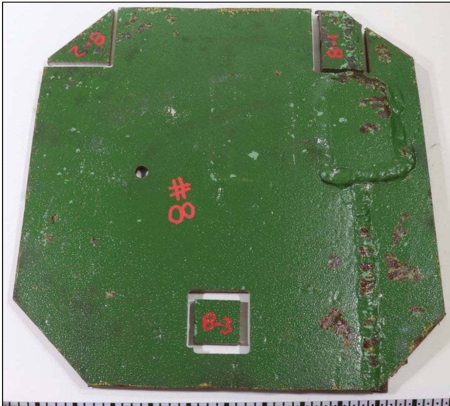
Figure 142. An image of the exterior surface of Coupon 8 after CO 2 blast cleaning.
