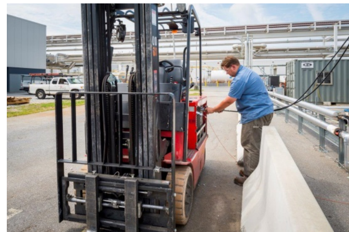
“First ever” fueling of fuel cell product (MHE) of hydrogen reformed from landfill gas. Testing showed no difference in stack performance vs. delivered H 2 source.
