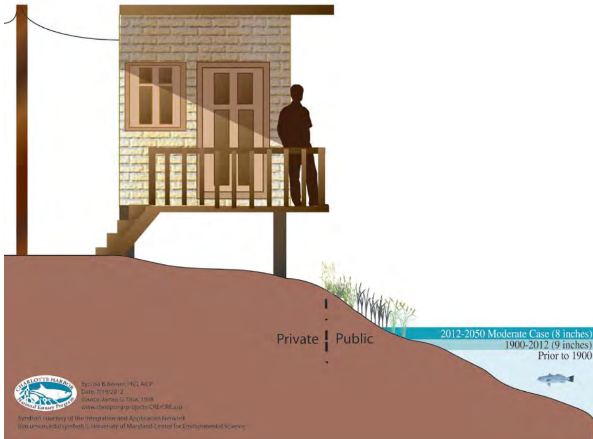
Figure 183: Rolling easement step 2: Year 2050. Moderate case 9 inches sea level rise. Mangroves and marsh move inland. Former mangroves become inundated.
