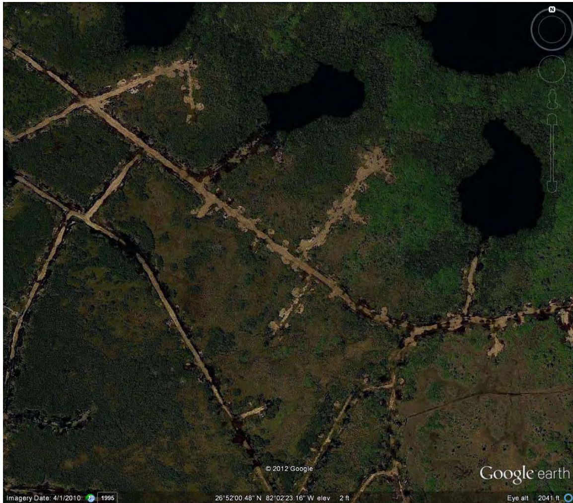
Figure 193: Restored backfilled mosquito control ditches on the Charlotte Harbor Preserve State Park. Source: Google Earth 2010
