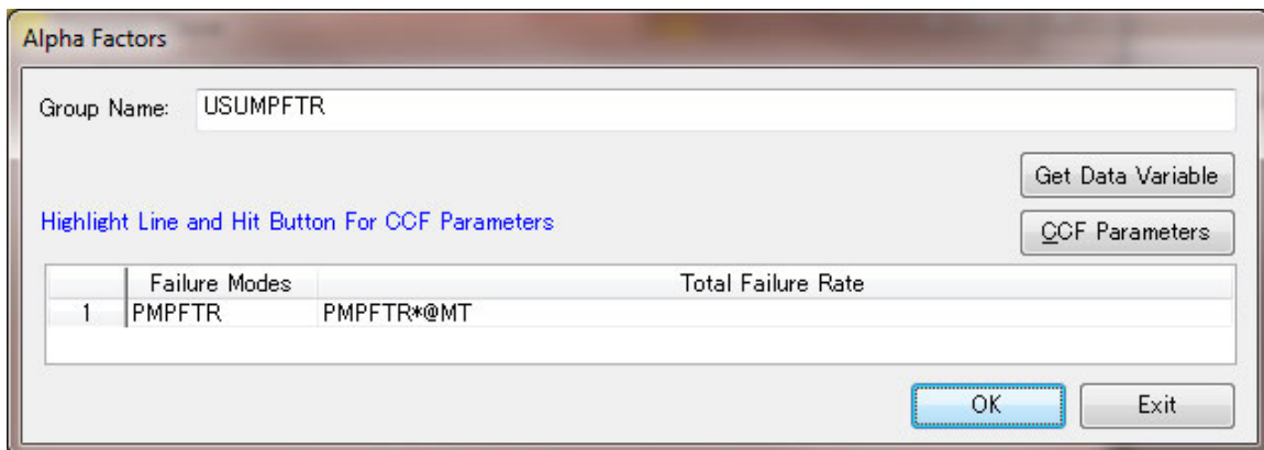
Figure 7-45. USUMP Common Cause Fail to Run Failure Mode and Failure Rate Equation
