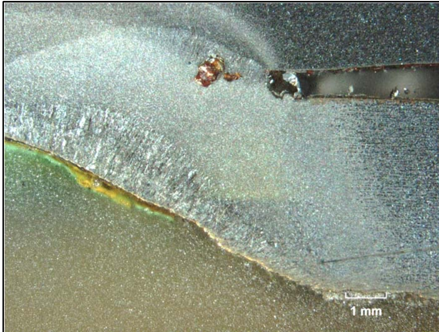
Figure 211. The left-hand feature in Figure 210 is shown at higher magnification. The weld indication (arrow) appeared to be an area of porosity.
