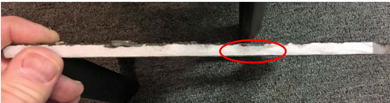
Figure A-3. The same area is shown after sandblasting on 3/20/19. A slight shadowing was observed in the area-of-concern, but no corrosion product was noted.
