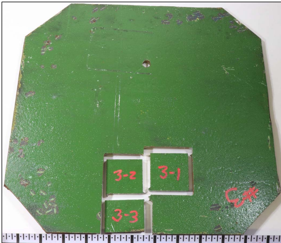
Figure 134. An image of the exterior surface of Coupon 3 after CO 2 blast cleaning.
