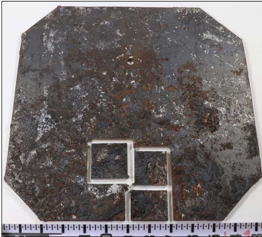
Figure 133. An image of the interior surface of Coupon 3 after CO 2 blast cleaning.
