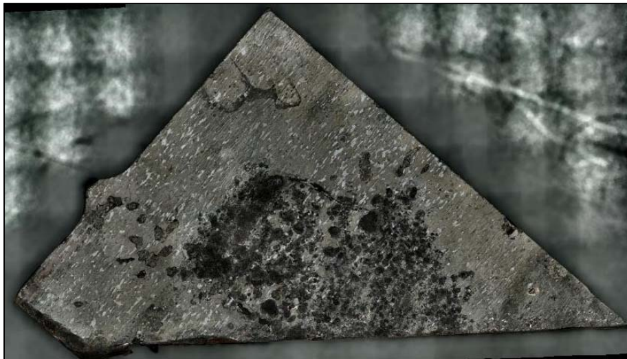
Figure 172. A screenshot of the 3D digital image of a specimen excised from Coupon 10 labeled as 10-2, after CO 2 blast cleaning
