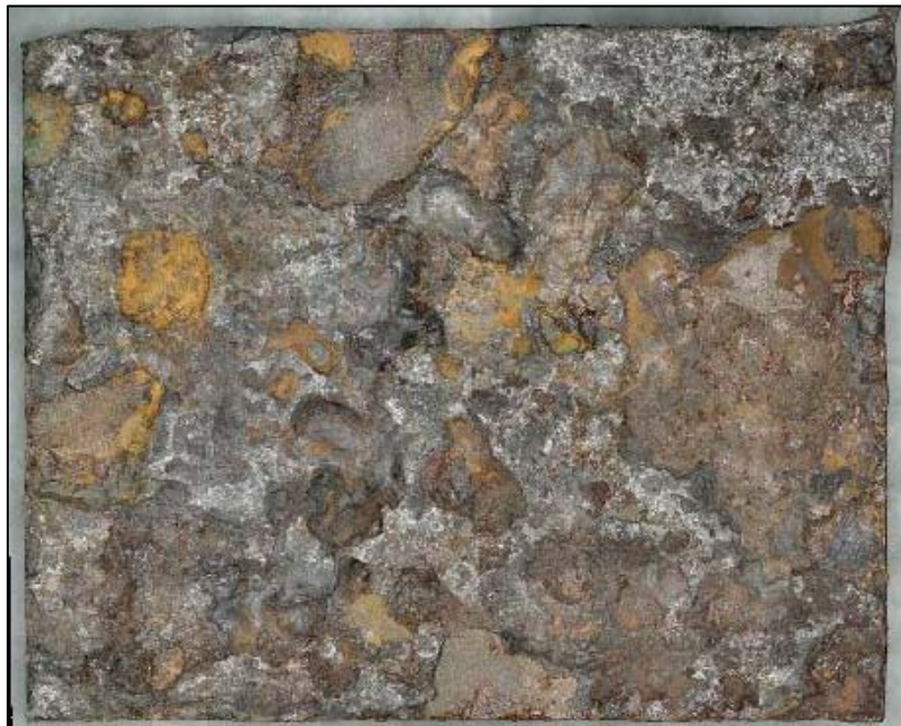
Figure 166. A screenshot of the 3D digital image of a specimen excised from Coupon 7 labeled as 7-3, after CO 2 blast cleaning
