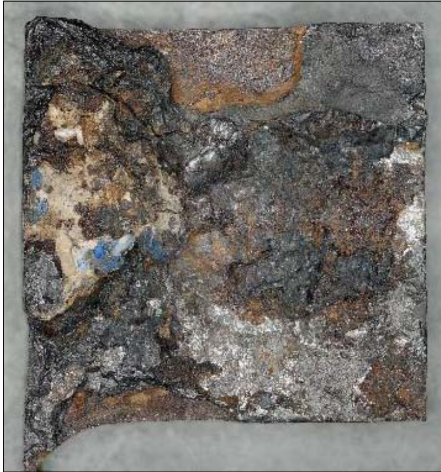
Figure 167. A screenshot of the 3D digital image of a specimen excised from Coupon 7 labeled as 7-4, after CO 2 blast cleaning
