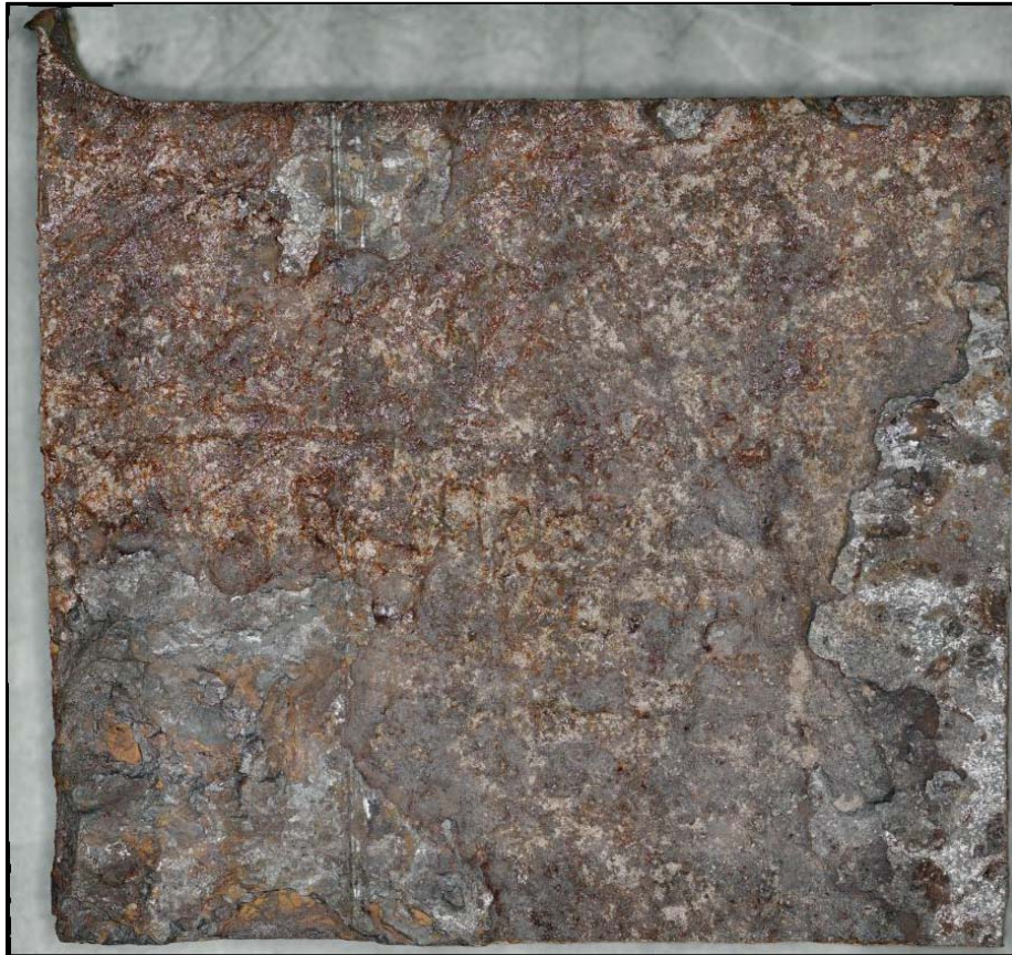
Figure 161. A screenshot of the 3D digital image of a specimen excised from Coupon 6 labeled as 6-1, after CO 2 blast cleaning
