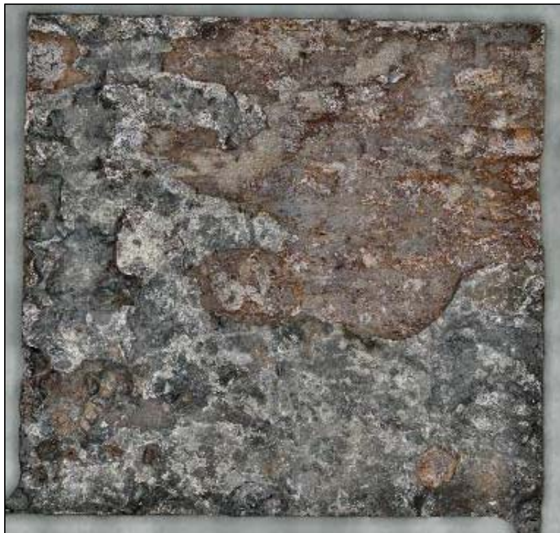
Figure 156. A screenshot of the 3D digital image of a specimen excised from Coupon 3 labeled as 3-2, after CO 2 blast cleaning
