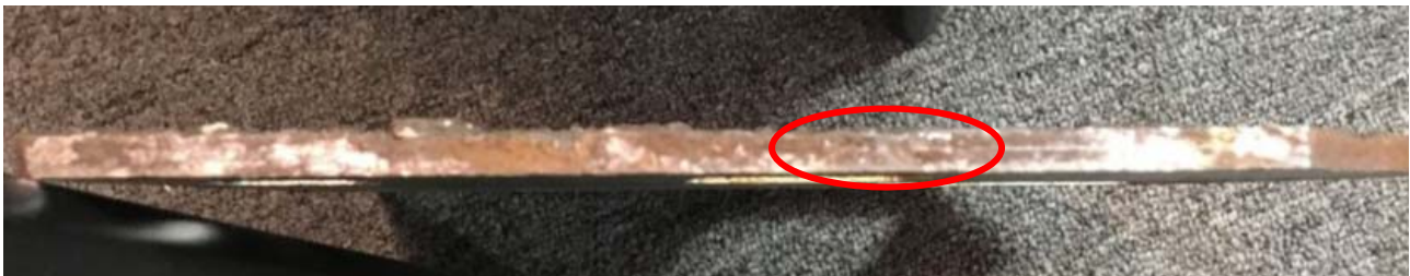
Figure A-2. The same edge of Coupon #7 is shown on 3/20/19 after laboratory testing by IMR and subsequent storage. The red circle corresponds to the same area shown in Figure A-1. Note that the left ~1/4 of the coupon was consumed for mechanical testing, etc., but the area-of-concern remained intact.
