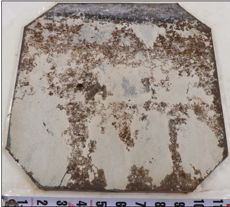
Figure 28. An image of the interior surface of Coupon A2 in the as-received condition.
