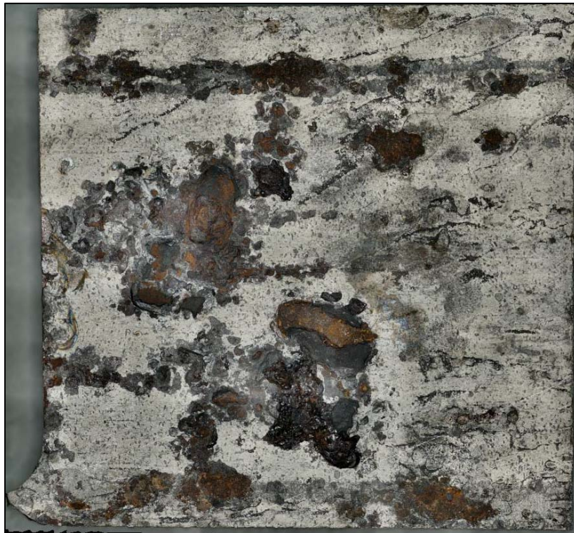
Figure 150. A screenshot of the 3D digital image of a specimen excised from Coupon 1 labeled as 1-2, after CO 2 blast cleaning
