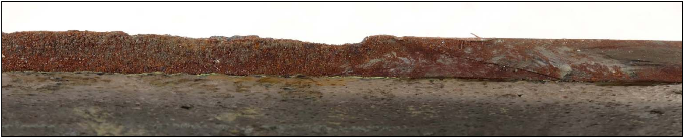
Figure 27. An image of a representative edge of Coupon A1 in the as-received condition.
