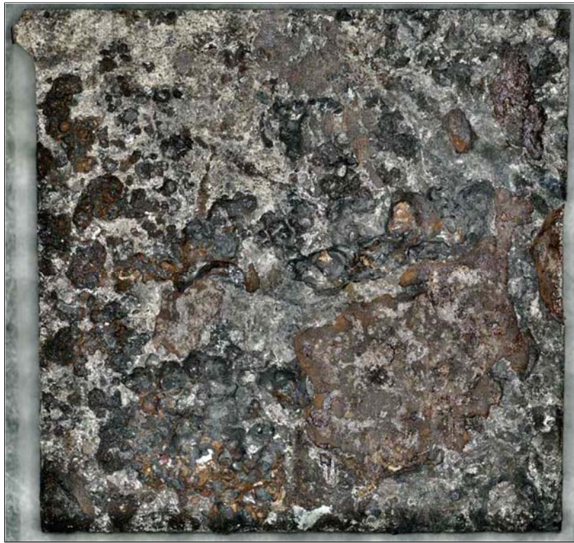
Figure 155. A screenshot of the 3D digital image of a specimen excised from Coupon 3 labeled as 3-1, after CO 2 blast cleaning
