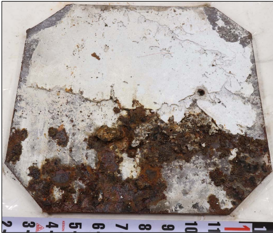
Figure 25. An image of the interior surface of Coupon A1 in the as-received condition.
