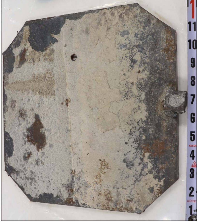
Figure 10. An image of the interior surface of Coupon 5 in the as-received condition.
