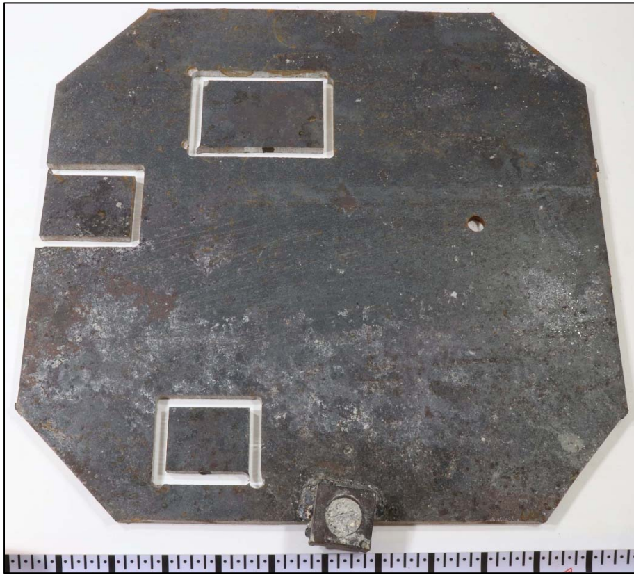
Figure 135. An image of the interior surface of Coupon 5 after CO 2 blast cleaning.
