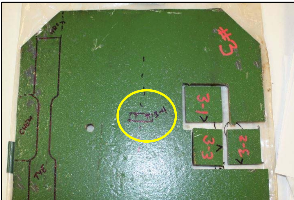
Figure B-2. Coupon #3 photograph showing the location of metallographic specimen 3-4 in relation to 3-1, 3-2 and 3-3.
