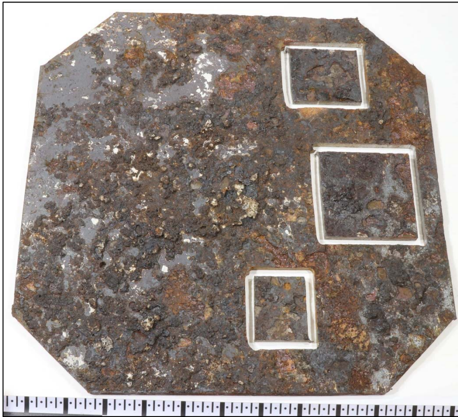
Figure 139. An image of the interior surface of Coupon 7 after CO 2 blast cleaning.
