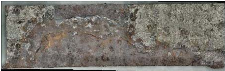
Figure 154. A screenshot of the 3D digital image of a specimen excised from Coupon 2 labeled as 2-3, after CO 2 blast cleaning
