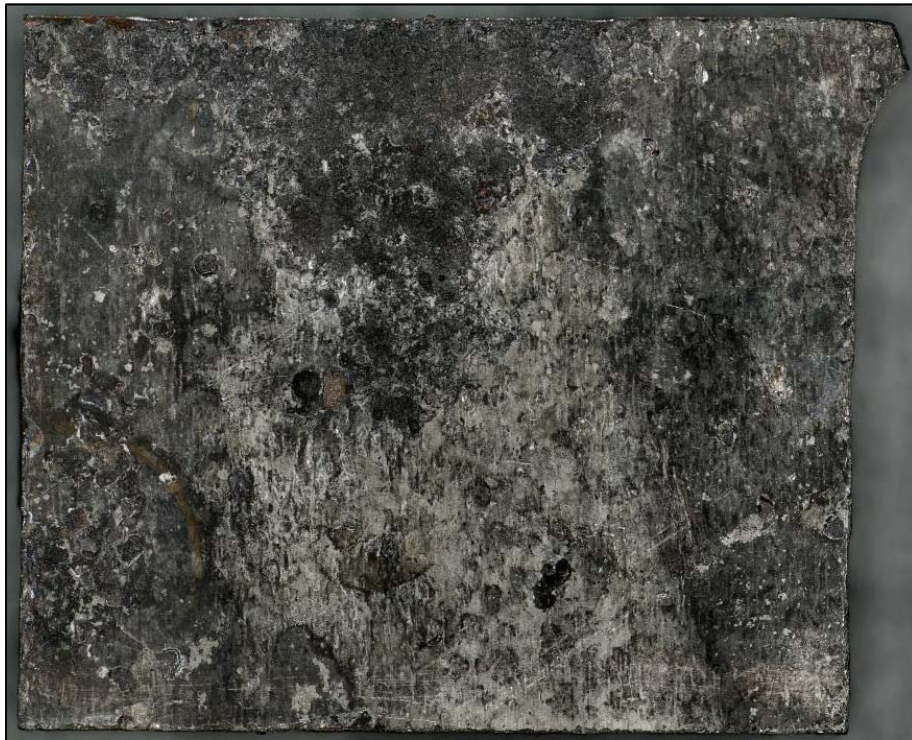
Figure 171. A screenshot of the 3D digital image of a specimen excised from Coupon 10 labeled as 10-1, after CO 2 blast cleaning
