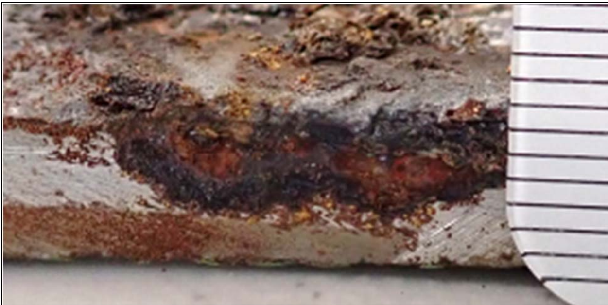
Figure A-5. The same area is shown in an image provided prior to shipping Coupon #7 to IMR (provided to IMR on March 13, 2019). What appeared to be a deep corrosion pit was actually rust-colored staining of the edge surface
