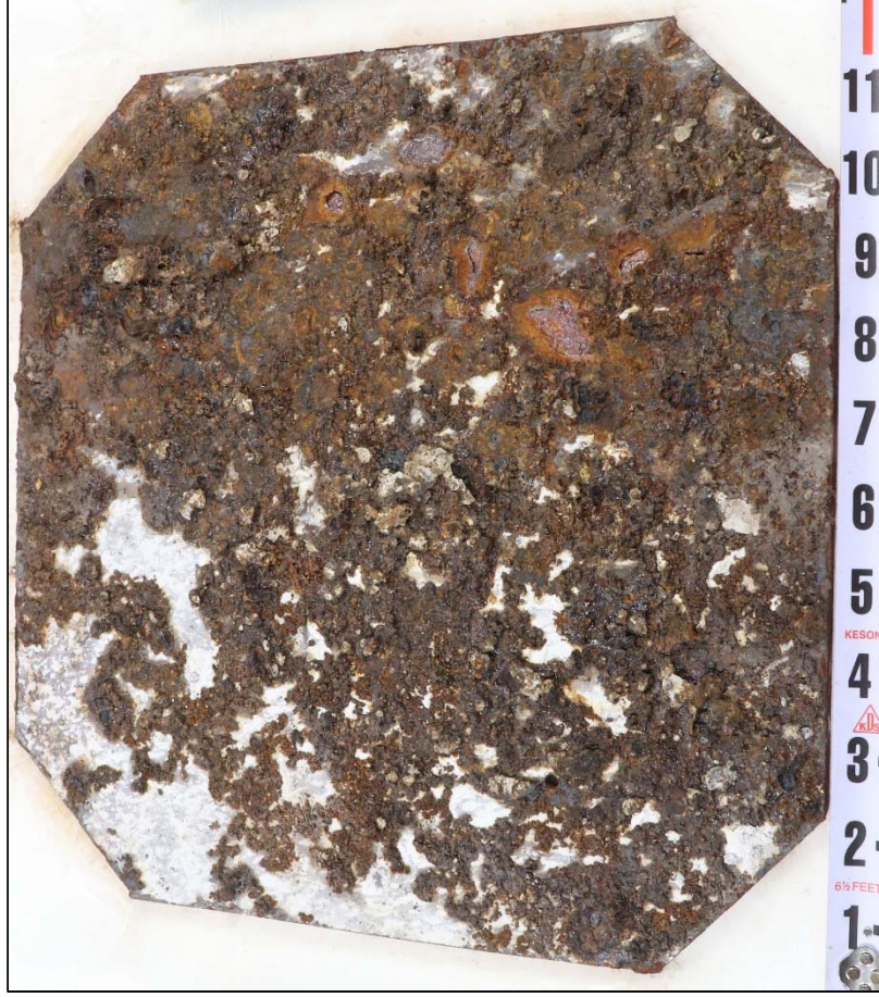
Figure 16. An image of the interior surface of Coupon 7 in the as-received condition.
