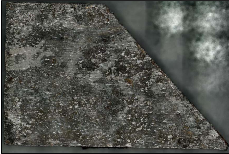
Figure 173. A screenshot of the 3D digital image of a specimen excised from Coupon 10 labeled as 10-3, after CO 2 blast cleaning
