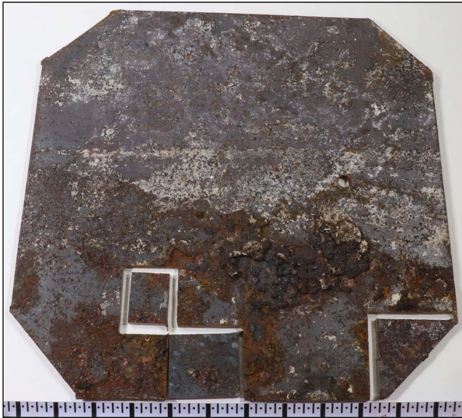
Figure 145. An image of the interior surface of Coupon A1 after CO 2 blast cleaning.
