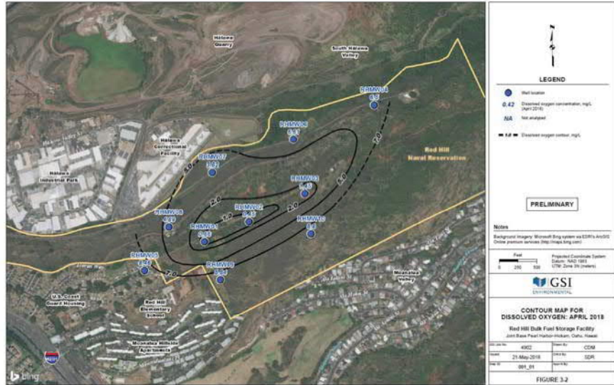
Figure 3-2: Contour Plot of O 2 Concentrations from the Facility Groundwater Monitoring Network (April 23-25, 2018)
