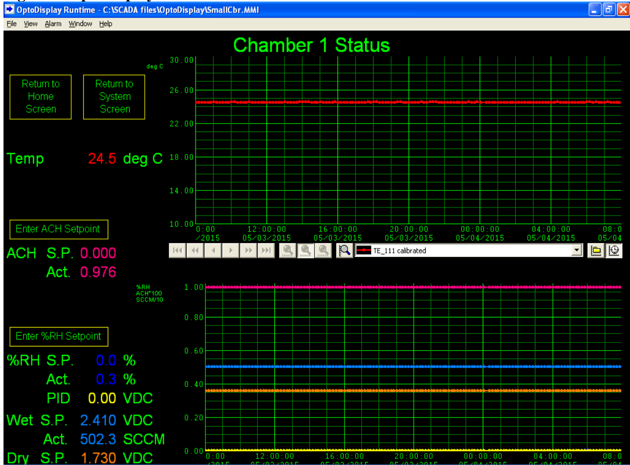
Figure 2. OptoDisplay Runtime Chamber Status Screen
