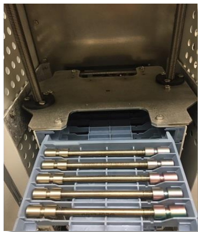
Figure 10. Loading the sample tray into the TD when full.
