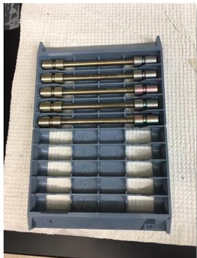
Figure 9. Loading sorbent tubes into the TD 50:50 tube tray.
