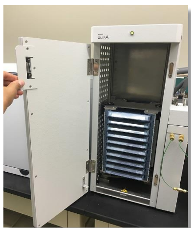
Figure 8. Opening the TD 50:50 door to access tube trays.
