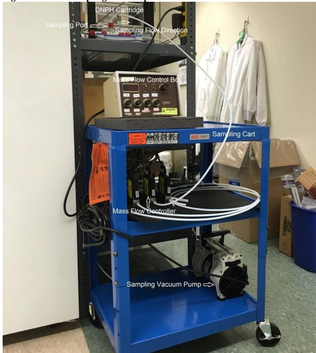
Figure 3. DNPH sampling cart setup
