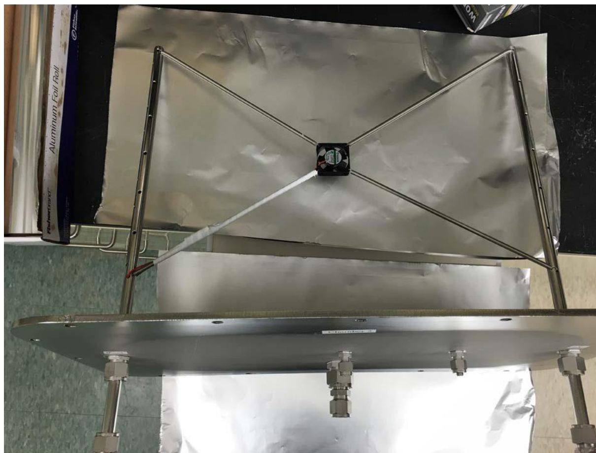
Figure 3. Picture of Mixing Fan setup
