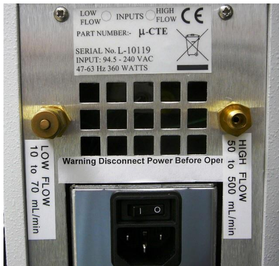
Figure 5-2 \mu -CTE gas inlets – Left low-flow and Right high-flow and power connection and switch
