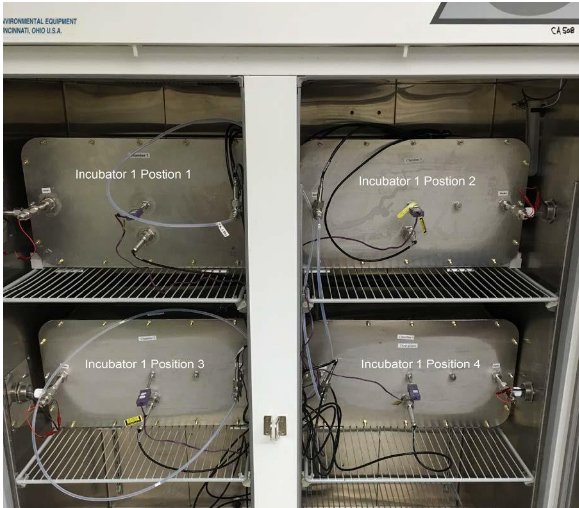
Figure 4. Incubator 1 with Chamber Locations
