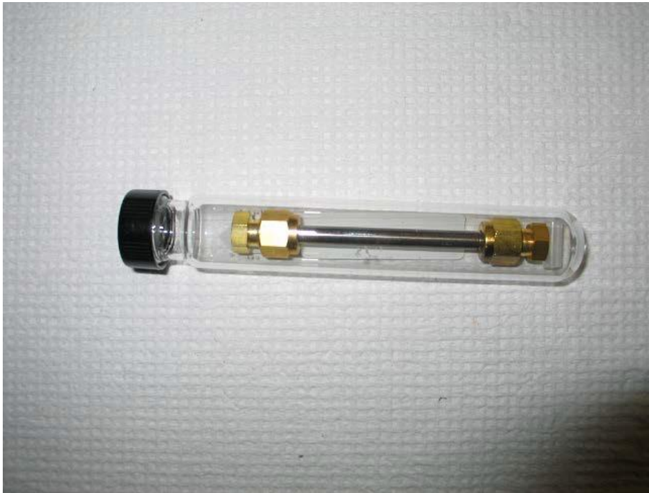
Figure 4. Carbopack™ X Sampling Tube in Capped Glass Culture Tube
