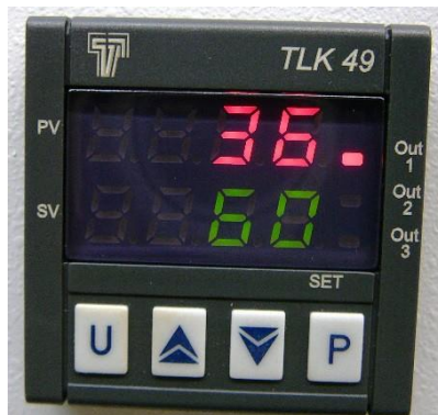
Figure 5-3 Temperature controller interface
