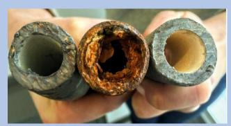
Lead is not naturally found in water. Lead from lead pipes, faucets, and fixtures can dissolve into water or sometimes can enter as flakes or small particles.
