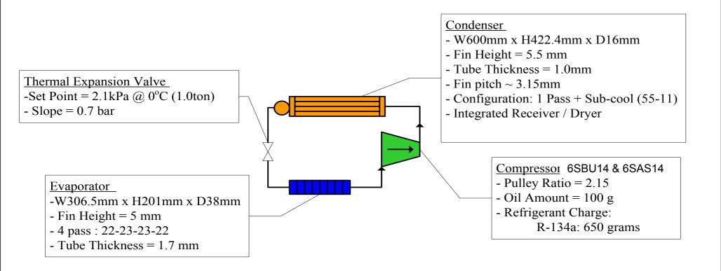
All components were common during testing of the 6SB\*14 and 6SAS14 compressors.
