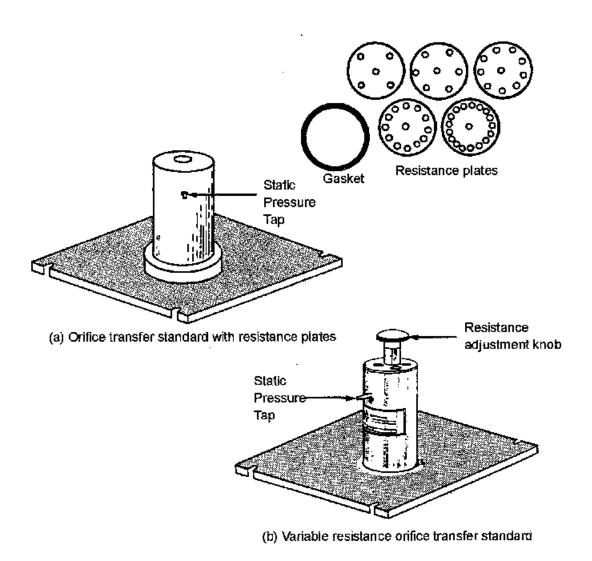
Figure 7. Typical orifice-type flow rate transfer standards.
