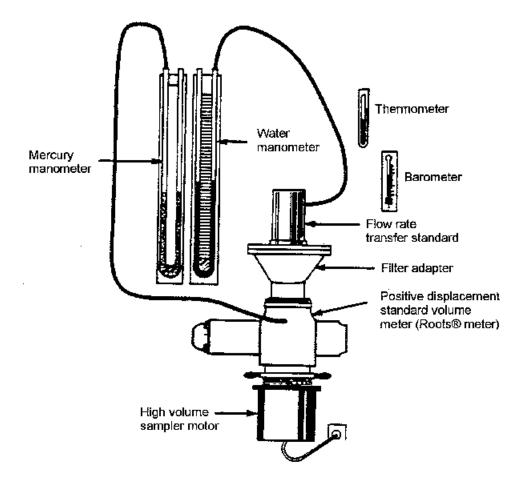
Figure 6. Flow rate transfer standard calibration setup.
