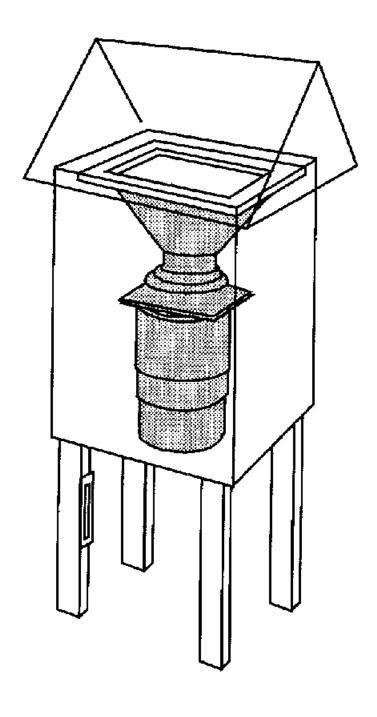
Figure 1. High-volume sampler with shelter.
