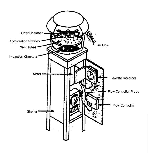
Figure 3. High-volume sampler with mass flow controller and impactor design size select inlet.
