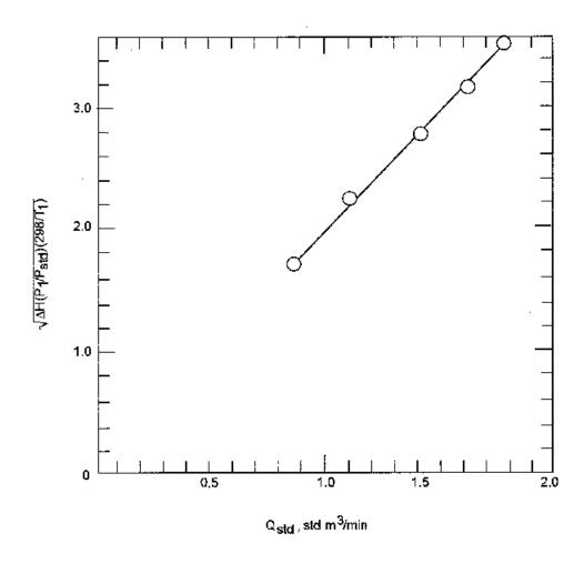
Figure 9. Typical calibration curve for a flow rate transfer standard.
