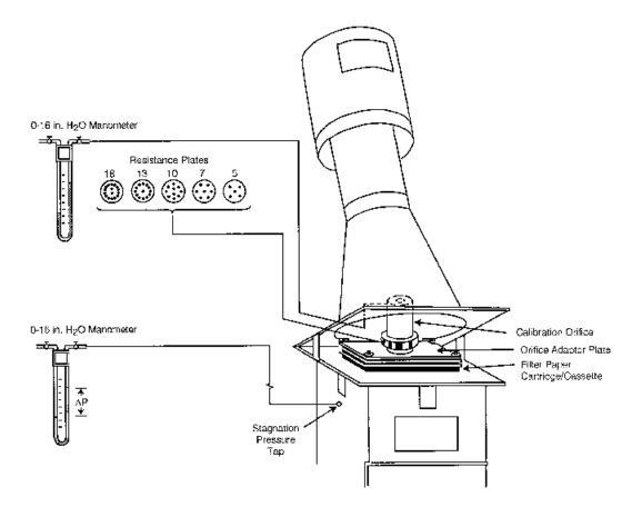
Figure 12. Calibration of a typical volumetric flow controller (VFC).
