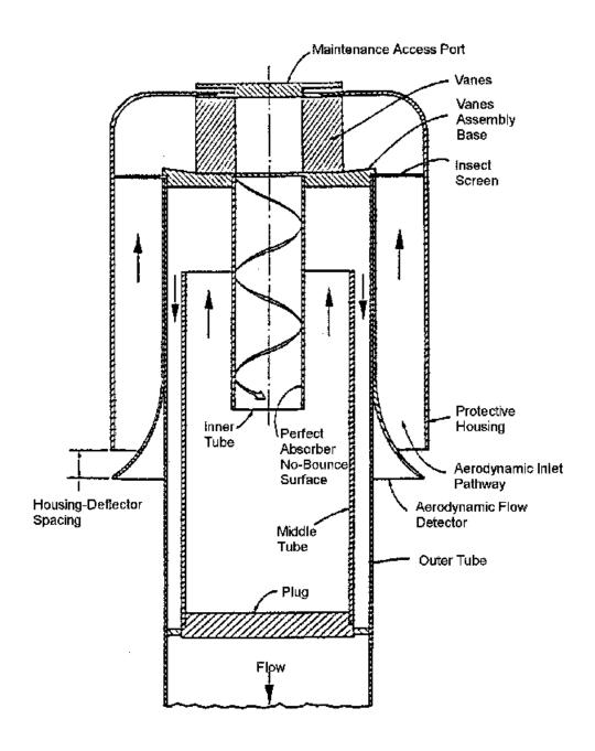
Figure 5. Schematic diagram of a cyclonic inlet for size select sampling for particulate matter.
