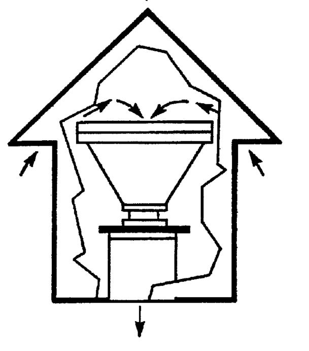
Figure 2. Inlet to EPA approved high volume sampler.
