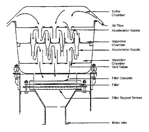
Figure 4. Schematic diagram of an impaction inlet for size select sampling for particulate matter.
