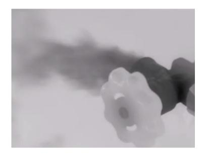
The Ventus Optical Gas Imaging Camera can detect small (~60 g/hr) leaks from several meters away or large leaks from hundreds of meters away. Detection as low as 6g/hr depending on distance, focal length of lens, delta T between gas and background temperatures and environmental conditions such as sun, clouds, wind, rain, fog, sleet and snow.
