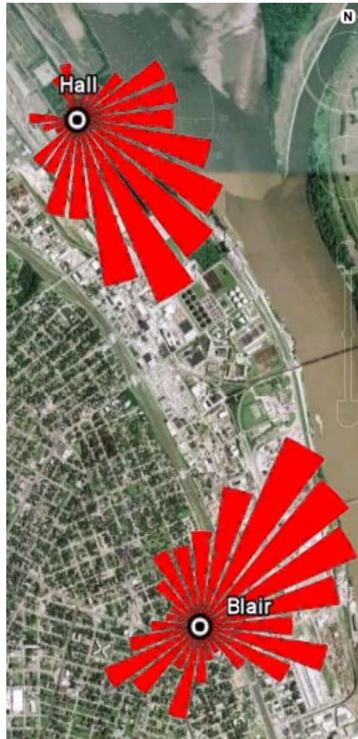
Figure 4-10. Conditional probability function (CPF) plots for the PM 10 selenium excess concentration distributions at Blair and Hall sites using hourly surface winds from St. Louis Lambert International Airport.
