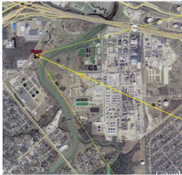
Figure 16: Resultant wind direction plot for Site B at 07:00 10/01/07 (CST)
