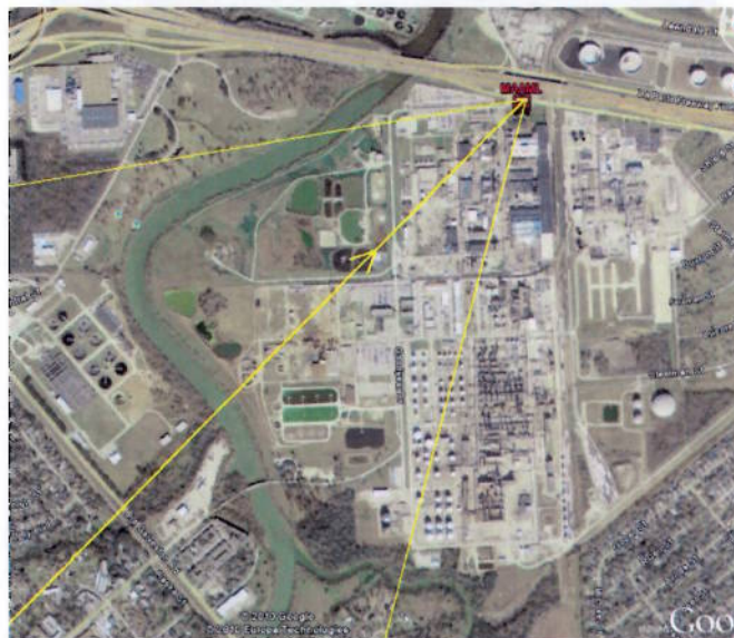
Figure 11: Resultant wind direction plot at 12:00 09/07/07 (CST)
